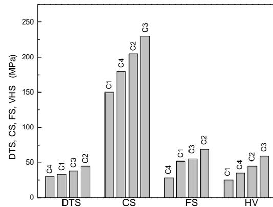
Fig. 1. Diametral tensile strength (DTS), compressive strength (CS), flexural strength (FS) and Vickers hardness (HV) of investigated dental composites.
