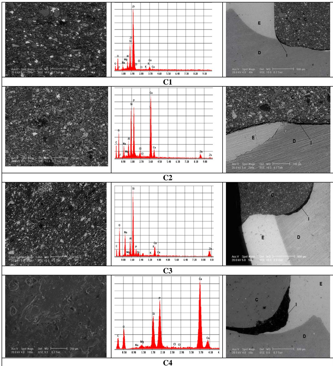
Fig. 2. SEM images of dental composites (left), their EDX spectra (middle) and SEM images of composite / tooth hard tissue interface (right, C-composite, D-dentine, E-enamel, I-interface).
