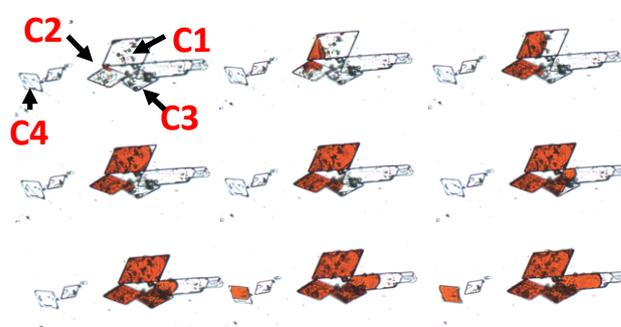
Fig. 5. The phase transformation of metastable  $\beta$ -HgI<sub>2</sub>  $\rightarrow$   $\alpha$ -HgI<sub>2</sub>
