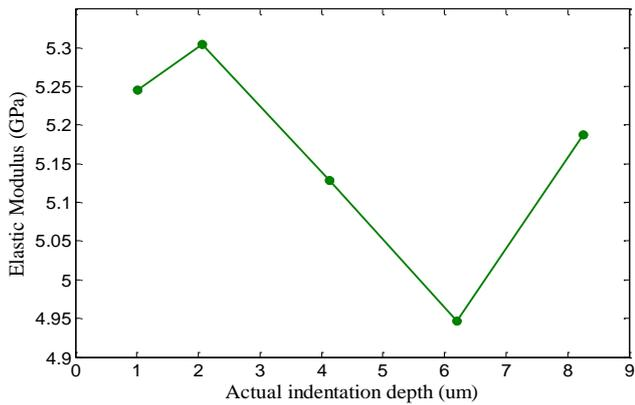
Fig. 5. The relationship between elastic modulus and indentation depth.
