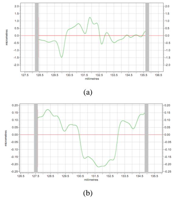
Fig. 9. The form accuracy (a) surface before turning (b) surface after turning.
