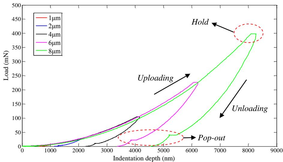
Fig. 3. The relation curve between load and displacement for PEEK.
