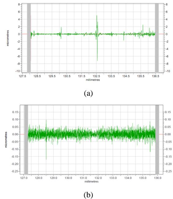
Fig. 10. The surface roughness (a) surface before turning (b) surface after turning.
