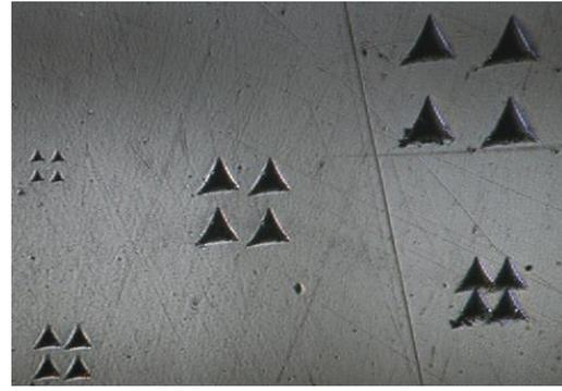
Fig. 2. The micro-photograph of indentation for PEEK.
