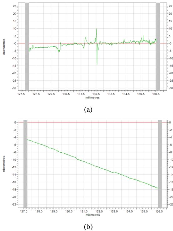
Fig. 8. The surface profiles (a) surface before turning (b) surface after turning.
