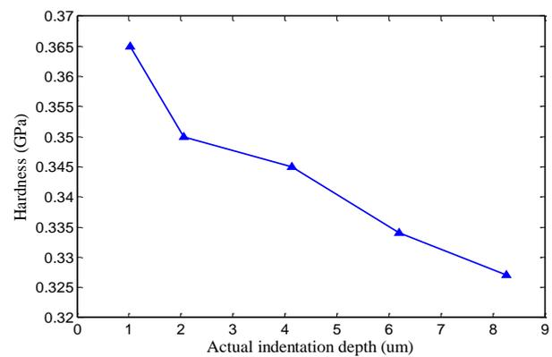
Fig. 4. The relationship between nano-indentation hardness and indentation depth.
