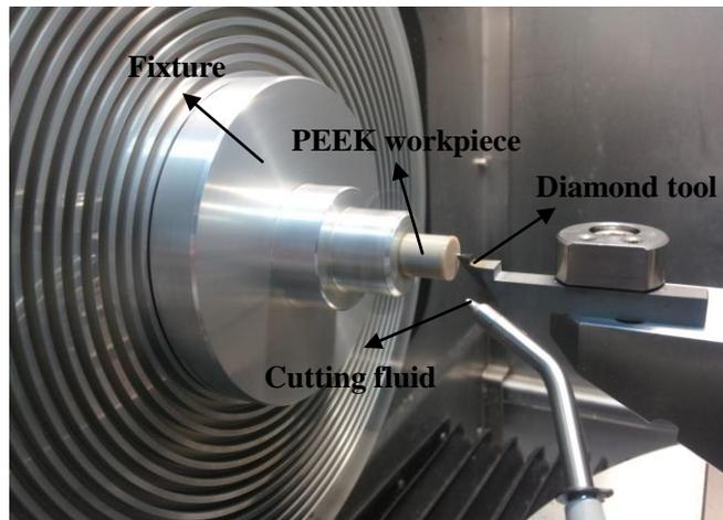
Fig. 6. The main section of the SPDT setup.
