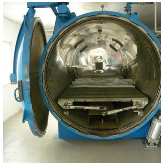
Fig. 1. Curing autoclave from Belco Avia Ltd.
