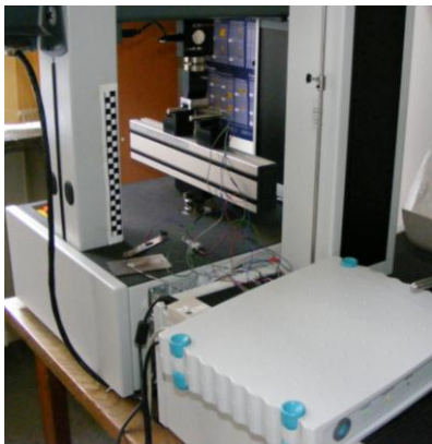
Fig. 1. Specimen connected to SPIDER8 device.
