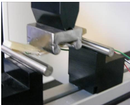
Fig. 2. Epoxy/4CSM450 specimen subjected to four-point bend test.
