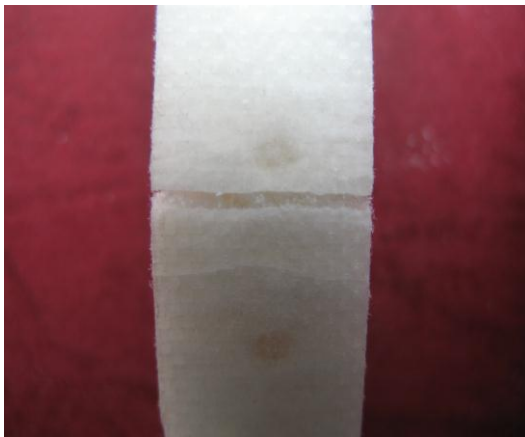
Fig. 10. Break detail of 4 mm thick nonwoven polyester mat subjected to three-point bend test.
