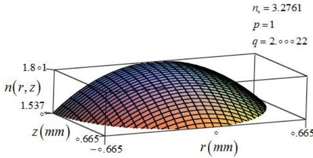
Fig. 4. Refractive index profile of planar microlens
