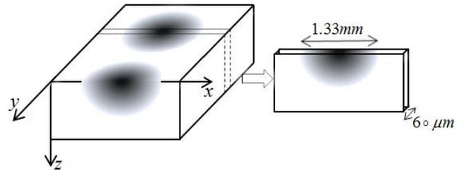
Fig. 2. Graded-index planar microlens and geometry of sample preparation
