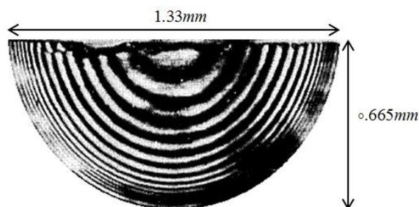
Fig. 3. The resulting interference pattern of planar microlens obtained by the total shear interferometer [11]
