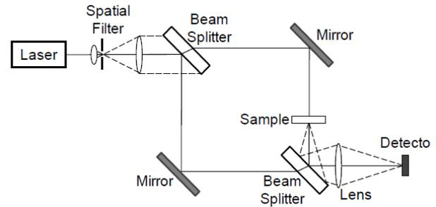
Fig. 1. Schematic of Mach-Zehnder interferometer used for measuring two dimensional refractive index profiles
