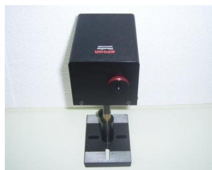
Fig. 2. Ophir WaveStar spectrometer.
