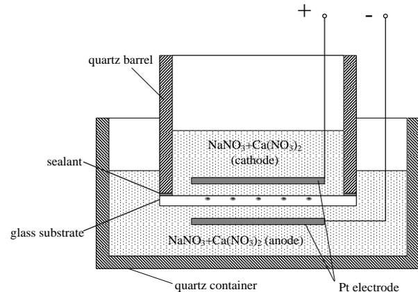
Fig. 2. Configuration of field-assisted ion-diffusion.
