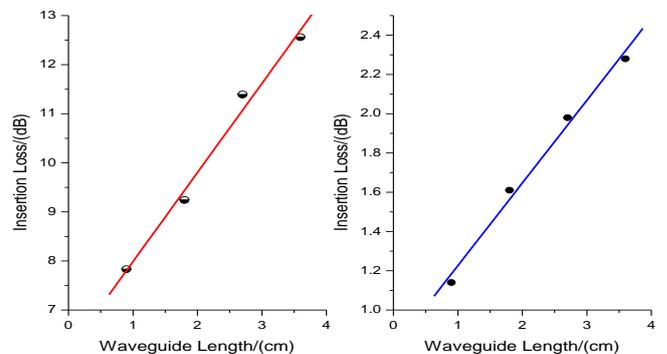
Fig. 5. Dependence of insertion loss of surface waveguide (left) and buried waveguide (right) on waveguide length.
