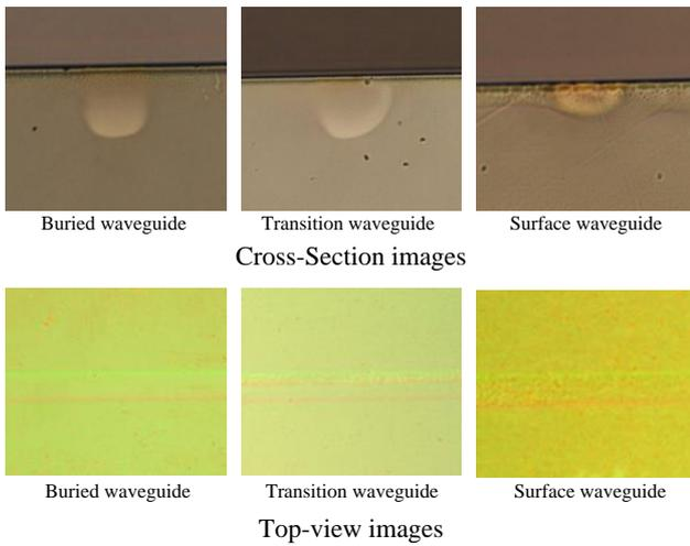
Fig. 3. Cross-section and top view of selectively buried channel waveguide at different portion.
