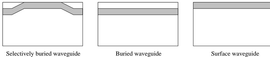
Fig. 4. Three types of waveguides fabricated on glass chip.
