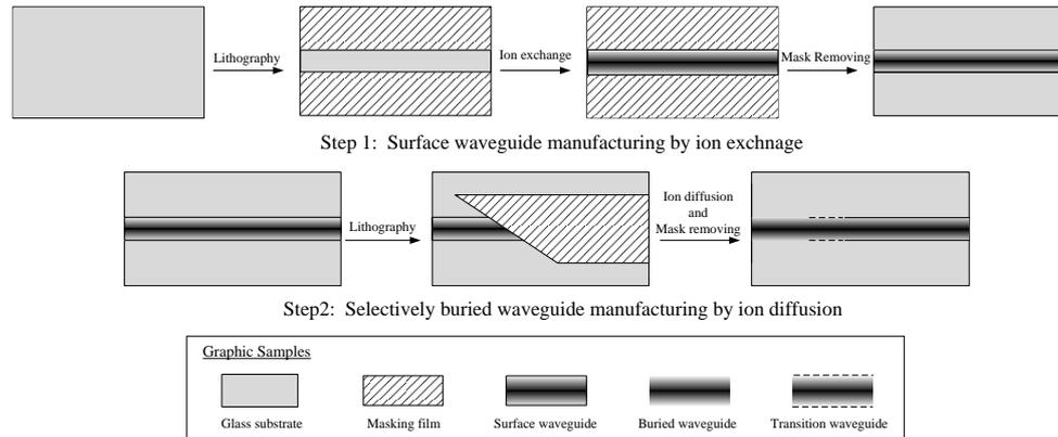
Fig. 1. Selectively buried channel waveguide manufacturing process.
