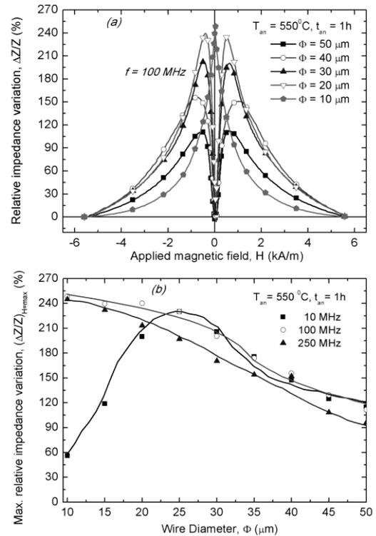
Fig. 2. Relative impedance variation,  $\Delta Z/Z = (Z - Z_{H=\text{max}})/Z_{H=\text{max}} * 100$  vs. applied magnetic field (a) and maximum relative impedance variation,  $(\Delta Z/Z)_{\text{max}}$  vs. wire diameter at different frequencies  $f$  (b) for the  $\text{Fe}_{73.5}\text{Si}_{13.5}\text{B}_9\text{Cu}_1\text{Nb}_3$  cold drawn wires annealed for one hour at  $550^\circ\text{C}$ .
