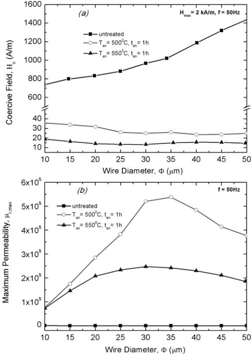
Fig. 1. Coercivity (a) and maximum value of the relative permeability (b) vs. wire diameter for the  $\text{Fe}_{73.5}\text{Si}_{13.5}\text{B}_9\text{Cu}_1\text{Nb}_3$  as-cast and cold drawn wires annealed for one hour at different temperatures.
