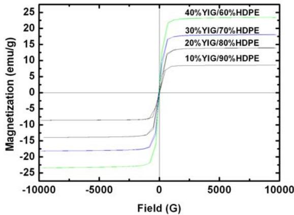
Fig. 1. Magnetic hysteresis loops of the composites with different volume fractions of YIG.
