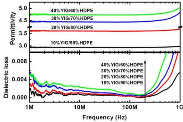
Fig. 4. Frequency dependence of the dielectric properties of the composite with different volume fractions of YIG.
