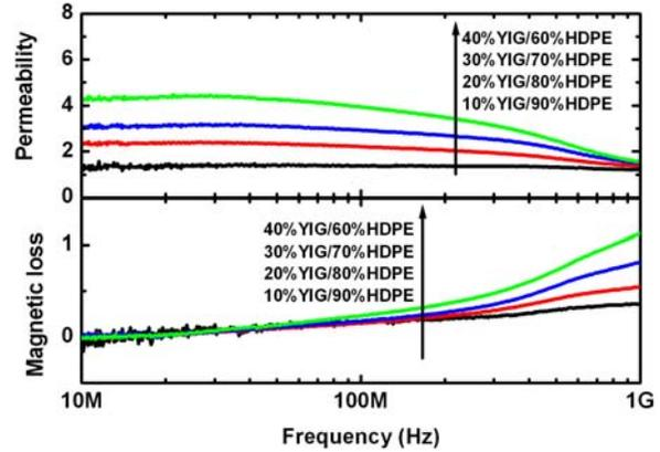
Fig. 2. Frequency dependence of the magnetic properties of the composite with different volume fractions of YIG.
