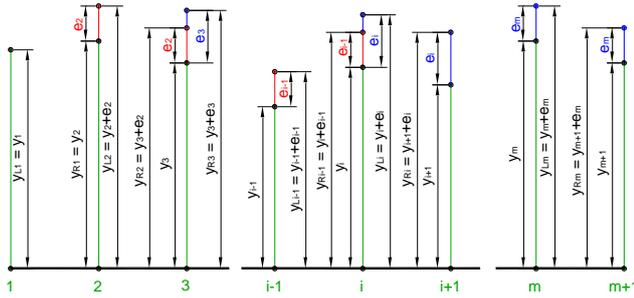
Fig. 2. True profile ( $y_i$ ) and measurements ( $y_{Ri}$  - right and  $y_{Li}$  - left).
