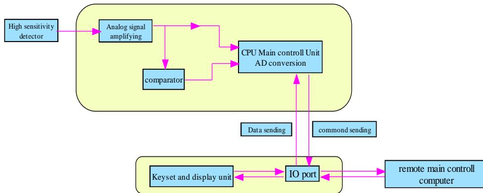
Fig. 4. Schematic circuit diagram of Analog to Digital Conversion (ADC) module
