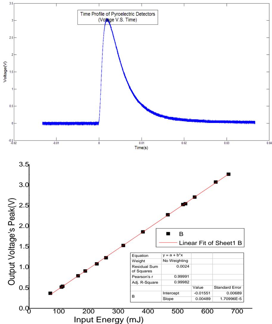
a) time profile of the output pulse b) Output Voltage's Peak Value versus Input Energy
