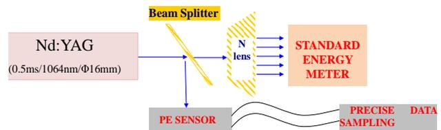
Fig. 1. Installation in the characteristics test experiment
