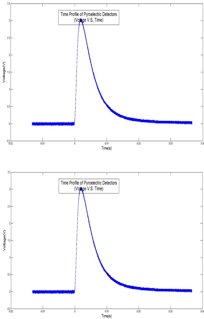
Fig. 3. Response curves of the PE detectors to different pulse width a) a 6 ns incident beam b) a 0.5 ms incident beam
