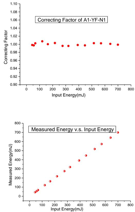
Fig. 6. Correcting Factor and Linearity of A1-YF-N1
