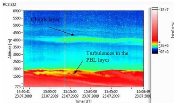
Fig. 2. RCS signal from LIDAR data generated by means of the Timisoara LIDAR, for the in 23.07.2009 episode, at Magurele location.
