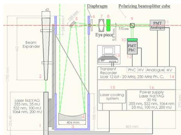
Fig. 1. Scheme of the Lidar system for the Timisoara system (in the frame of the ROLINET [7] and RADO [8] research projects).
