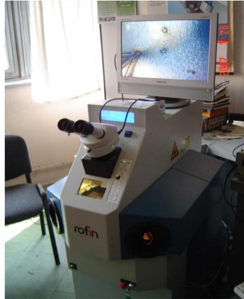
Fig. 2. ROFIN STARWELD laser installation
