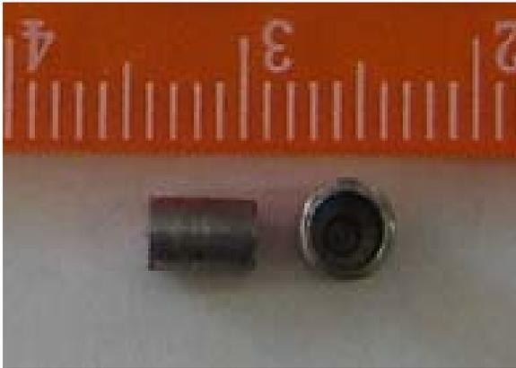
Fig. 1. Stainless steel microcapsules.
