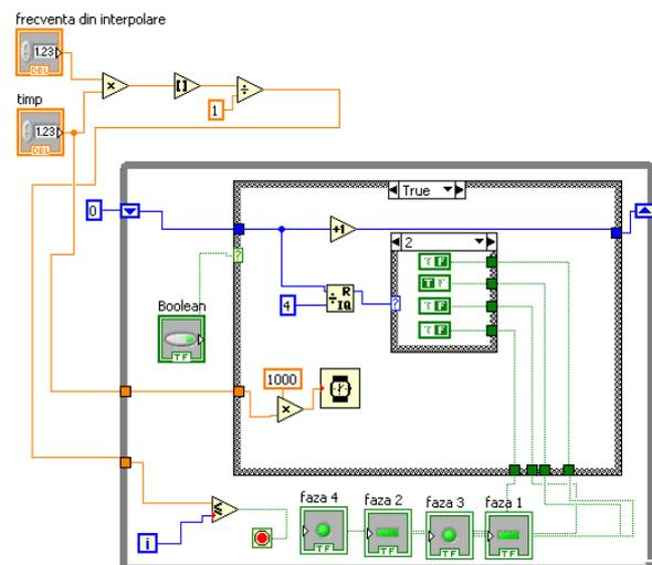
Fig. 9. The Block Diagram of the control software for the four phases of the electrical stepper motor.
