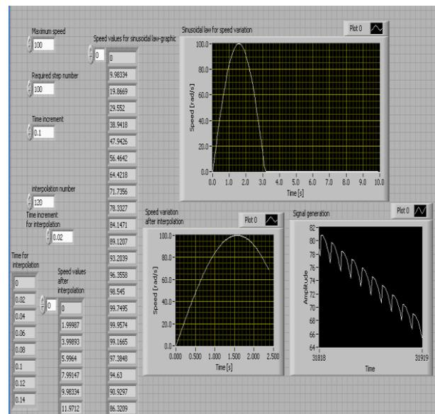
Fig. 8. The Front Panel of the control software.
