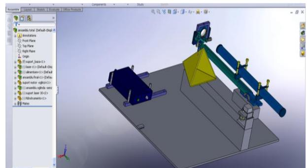
Fig. 3. The laser beam subassembly.
