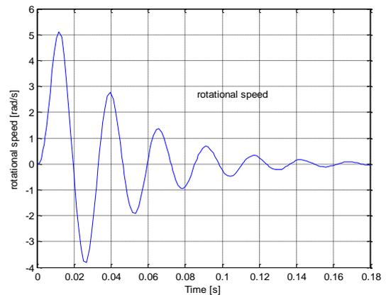
Fig. 6. Rotational speed dependence on time.
