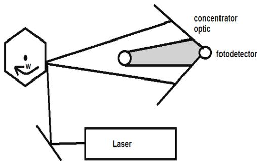
Fig. 1. Schematic of the system principle.
