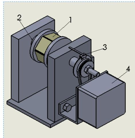
Fig. 2. The mirror and the electrical stepper motor subassembly.
