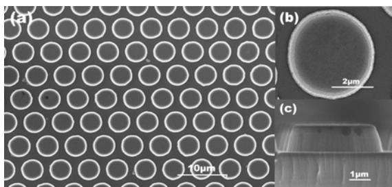
Fig. 1. Typical SEM images of the periodically patterned sapphire. (a) The surface morphology of the periodically patterned sapphire with low magnification (b) (c) Top-view and cross-sectional SEM image of the single unit.
