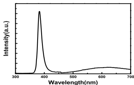
Fig. 4. Typical PL spectra of ZnO sunflower-like nanostructures using 266 nm laser as a source excitation.
