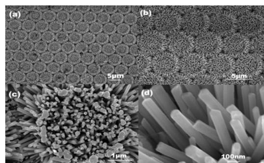
Fig. 3. FE-SEM images of ZnO (a) overall morphology at low resolution (5000 $\times$ ). (b)(c) High magnification image view of a typical sunflower-like ZnO on the top surface and sidewall.
