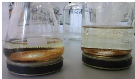
Fig. 10. Magnetically separation of the \gamma-Fe_2O_3 used as adsorbent for removal of Cr(VI) from aqueous solutions.
