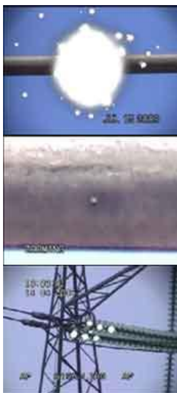
Corona on bus bar Corona source pinpointed - hole on bus bar Corona pinpointed on glass insulator
