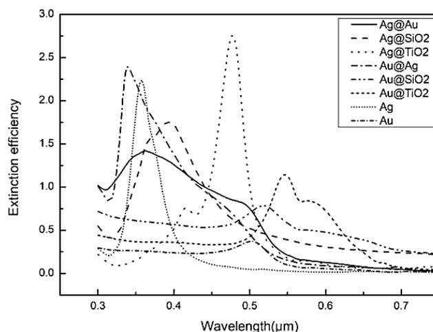
Fig. 2. Comparison of simulation results for various core–shell structures
