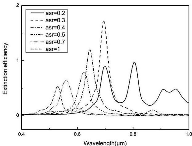
Fig. 6. Extinction spectra for different aspect ratios of the core-shell structure
