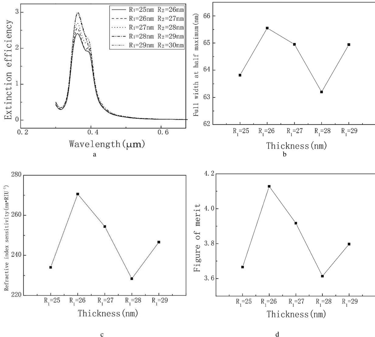
Fig. 4. Calculated results for  $\text{Ag@TiO}_2$  core-shell structures with fixed shell thickness ( $h = 1$  nm) and different core radii (25–29 nm): (a) extinction spectra; (b) full width at half maximum; (c) refractive index sensitivity distributions; (d) figure of merit
