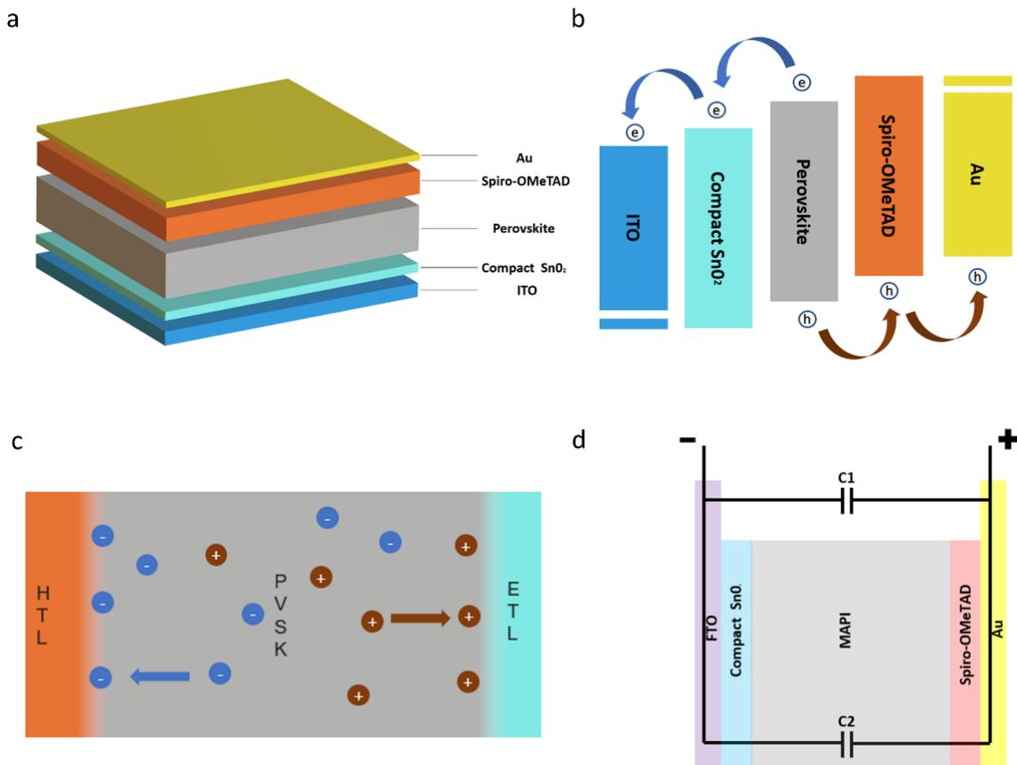
Fig. 3. (a) Structure of planar heterojunction perovskite solar cell, (b) Electron and hole movement in the cell, (c) Ion aggregation at the electron/hole transport layer boundary, (d) Simple electrical model of solar cell (color online)
