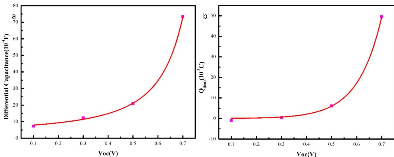
Fig. 7. (a) Differential capacitance values under different background light, (b) Total device charge values under different background light
