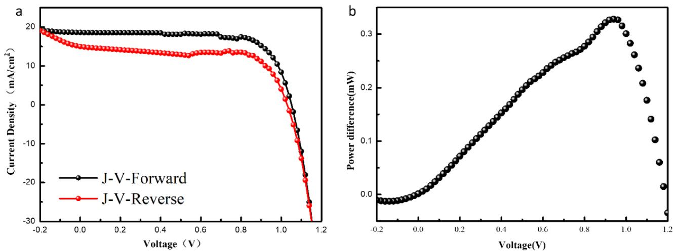
Fig. 2. (a) Cell forward and reverse sweep J-V curve, (b) Hysteresis power
