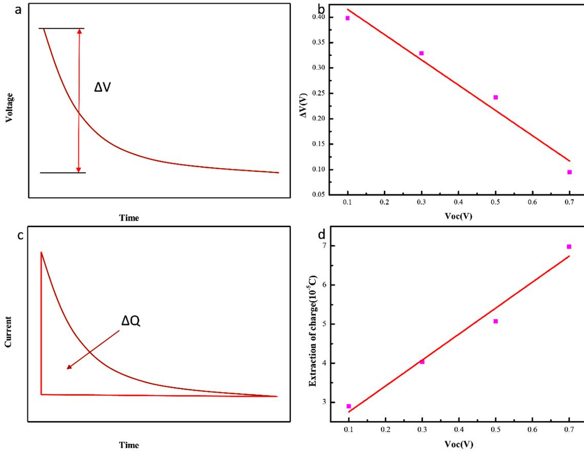
Fig. 6. (a) Schematic diagram of  $\Delta V$ , (b) Values of  $\Delta V$  for different  $V_{oc}$  conditions, (c) Schematic diagram of  $\Delta Q$ , (d) Extracted charge values under different  $V_{oc}$  conditions
