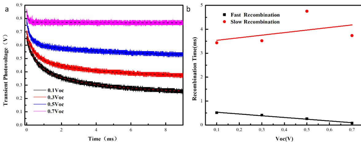
Fig. 4. (a) TPV test data and fitting results, (b) Charge recombination time (color online)
