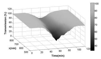
Fig. 2. Time and wavelength dependent transmission (%) change (t=0-60 min  $CO_2$ , t=60-120 min  $N_2$ )
