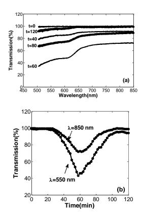
Fig. 3. a) Wavelength dependent light transmission change: bold lines corresponds to  $N_2$  medium, b) Comparison of the time dependent light transmission at wavelengths 550 nm and 850 nm (t=0-60 min CO<sub>2</sub>, t=60-120 min N<sub>2</sub>)
