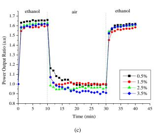
Fig. 5. Response and recovery rate of sensor with 0.8 mm waist diameter and (a) 1 cm, (b) 3 cm, (c)5 cm unclad length (color online)
