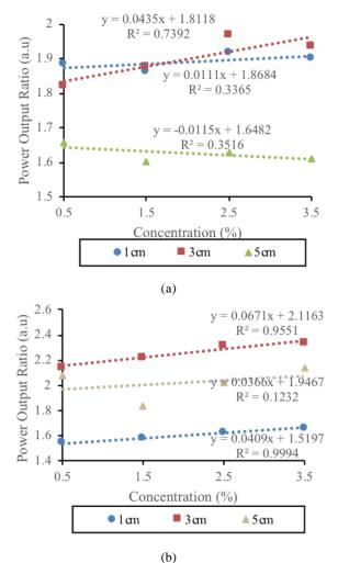
Fig. 6. Sensitivity of various unclad length with (a) 0.8 mm and (b) 0.5 mm waist diameter (color online)
