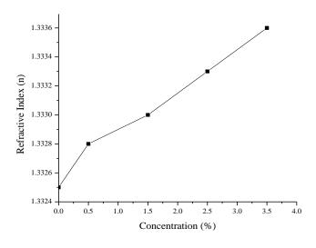
Fig. 3. Refractive index of varies ethanol concentration
