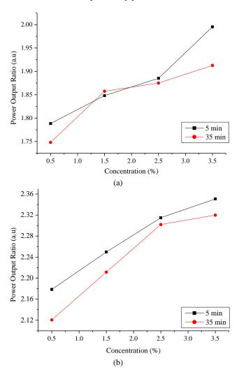
Fig. 7. Repeatability of 3 cm unclad length with (a) 0.8 mm and (b) 0.5 mm waist diameter POF (color online)
