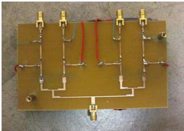
Fig. 4. Photo of actual PIN diode switching circuit.
