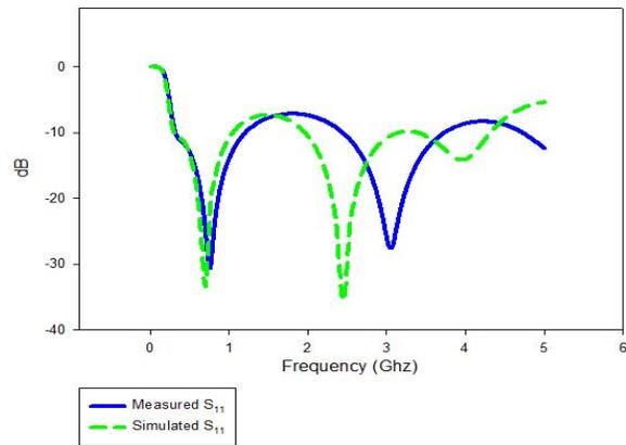
Fig. 10. Calculated return loss ( $S_{11}$ ) at switch ON mode.
