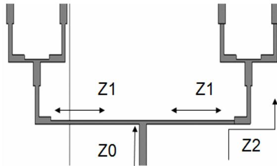
Fig. 2. T-junction power divider.
