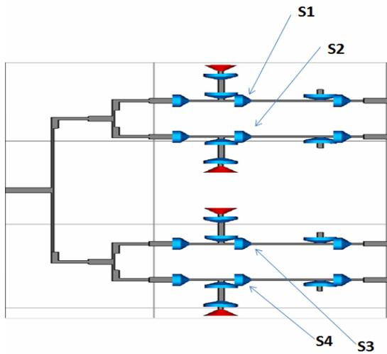
Fig. 3. PIN diode switching circuit incorporated with T-junction power divider.
