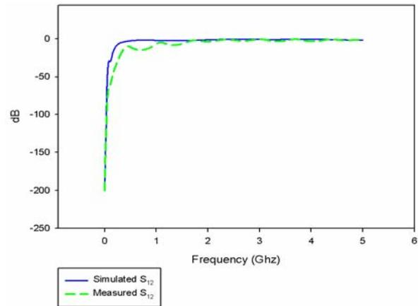
Fig. 11. Calculated transmission loss ( $S_{12}$ ) at switch ON mode.
