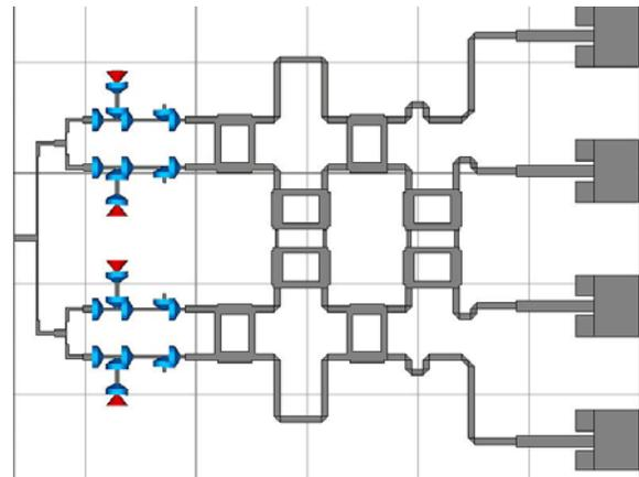
Fig. 5. Layout of integrated PIN diode switching circuit with Butler Matrix.
