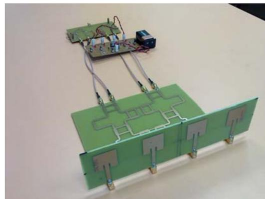
Fig. 6. Photo of integrated PIN diode switching circuit with Butler Matrix.
