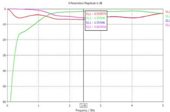
Fig. 8. Calculated return loss ( $S_{11}$ ) and transmission loss ( $S_{12}$ ) for switch OFF mode.
