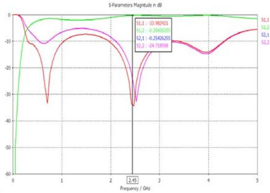
Fig. 7. Calculated return loss ( $S_{11}$ ) and transmission loss ( $S_{12}$ ) for switch ON mode.
