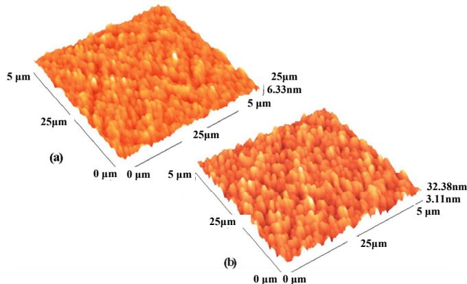
Fig. 2. Tapping mode AFM images of InN/AlN/kapton films deposited at 0.6 (a) and 0.8 Pa (b).
