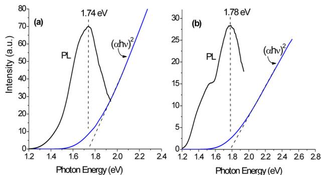
Fig. 3. Band gap estimation from PL spectra and Tauc's plot of InN films deposited at 0.6 (a) and 0.8 Pa (b)
