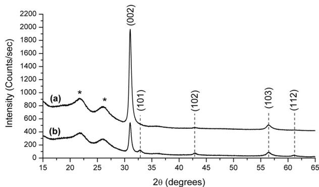
Fig. 1. XRD pattern of the as-deposited samples of InN grown on kapton substrate with AlN buffer in 0.6 (a) and respectively 0.8 Pa (b) of pure  $N_2$  atmosphere.
