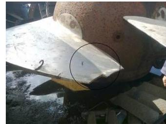
Fig. 2. Surface of the turbine blade from „CH 2 - Sample 2”
