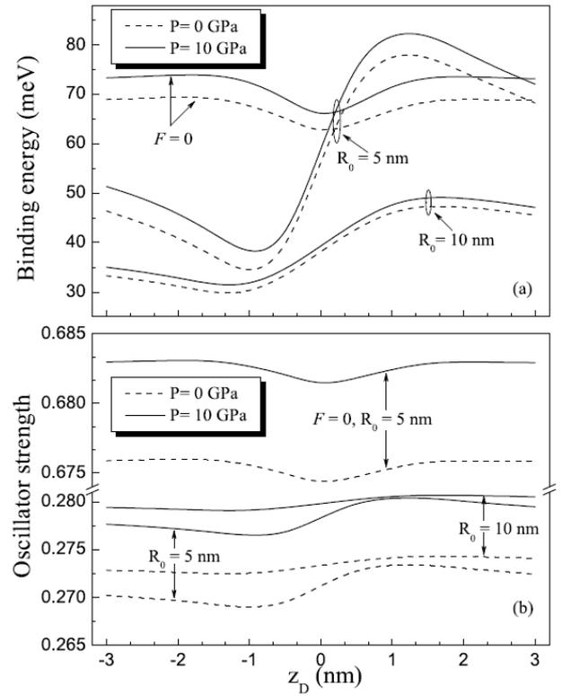
Fig. 2. The bound exciton binding energy (a) and the oscillator strength (b) as a function of the donor position  $z_D$  in cylindrical wurtzite  $\text{In}_{0.2}\text{Ga}_{0.8}\text{N}/\text{GaN}$  strained QD ( $H_0=2\text{nm}$ ) NWHETs with different QD radius under hydrostatic pressures. For the sake of comparison, the bound exciton binding energy without the BEF ( $F = 0$ ) has also been shown in (a).
