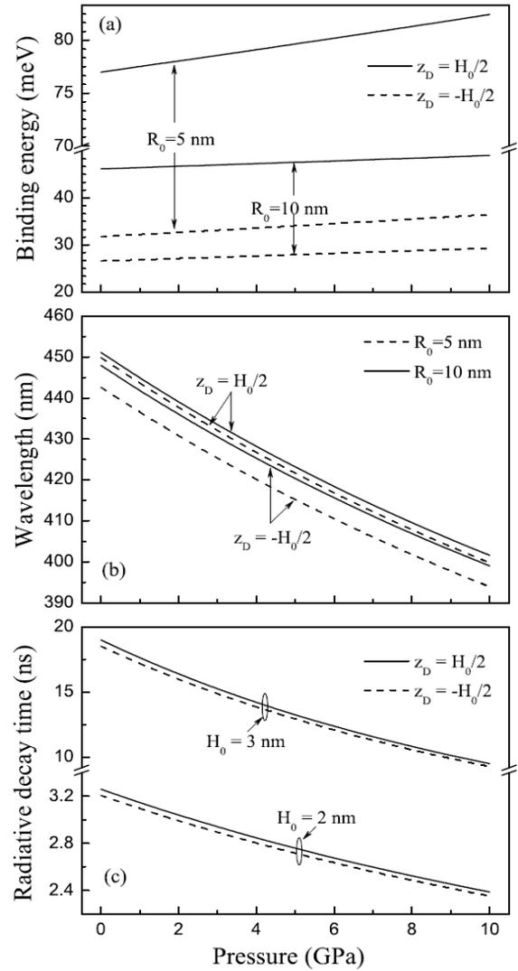
Fig. 1. The bound exciton binding energy (a), the emission wavelength (b) and the radiative decay time (c) as a function of the hydrostatic pressure  $P$  in cylindrical wurtzite  $\text{In}_{0.2}\text{Ga}_{0.8}\text{N}/\text{GaN}$  strained QD NWHTs. Here we choose the QD height  $H_0 = 2$  nm in (a) and (b) and the QD radius  $R_0 = 5$  nm in (c).
