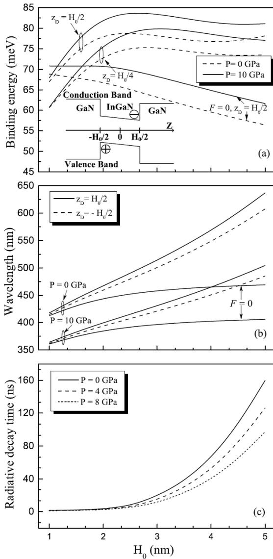
Fig. 3. The exciton binding energy (a), the emission wavelength (b) and the radiative decay time (c) as a function of the QD ( $R_0=5\text{nm}$ ) height  $H_0$  in cylindrical wurtzite  $\text{In}_{0.2}\text{Ga}_{0.8}\text{N}/\text{GaN}$  strained QD NWHTs under different hydrostatic pressures.
