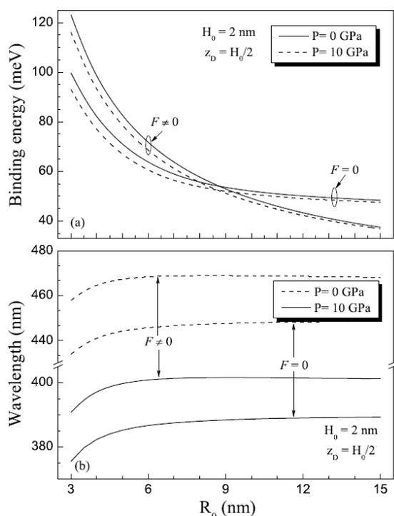
Fig. 4. The exciton binding energy (a) and the emission wavelength (b) as a function of the QD radius  $R_0$  in cylindrical wurtzite  $\text{In}_{0.2}\text{Ga}_{0.8}\text{N}/\text{GaN}$  strained QD NWHETs under different hydrostatic pressures.
