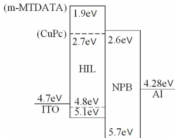
Fig. 3. Schematic energy level diagram for the hole-only devices.
