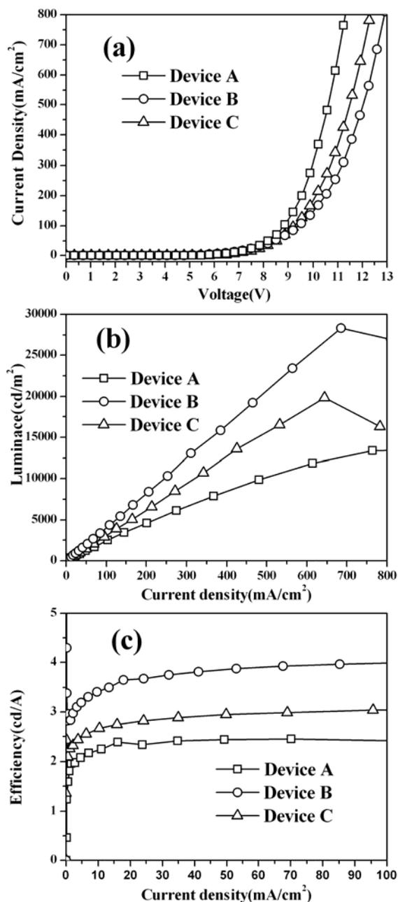
Fig. 1. (a) Current density - voltage, (b) current efficiency - current density, and (c) luminance - current density for devices A-C.
