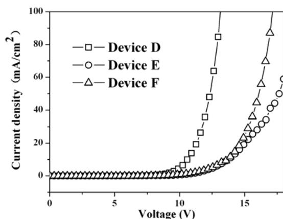
Fig. 4. Current density - voltage for the hole-only devices.
