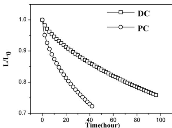
Fig. 5. Normalized luminance decay [luminance ( $L$ )/initial luminance ( $L_0$ )] vs. operating time for device B under DC and PC driving mode with 1:1 duty cycle, 50 Hz square wave and 5V reverse Voltage.
