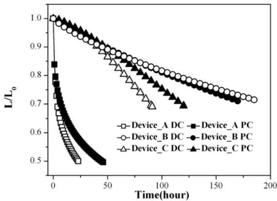
Fig. 2. Normalized luminance decay [luminance (L)/initial luminance (L<sub>0</sub>)] of devices A-C as a function of operating time for DC and PC operation with 1:1 duty cycle, 50 Hz square wave and 5V reverse Voltage.
