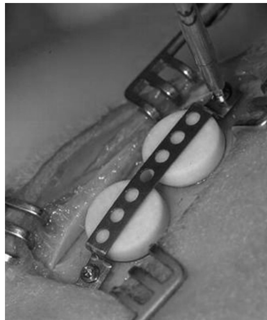
Fig. 2. Test implants were placed on the prepared sites on tibia bone in rabbits. To avoid influence of bone contact onto the vertical aspects of the implants during the tensile test, the implants were covered with Teflon® caps that were removed prior to the pull out procedure. The test surface of the implants were placed directly onto the prepared bone surface, and were left unaffected by the Teflon caps and the retention apparatus used to ensure good stability and contact between implant and bone during healing.
