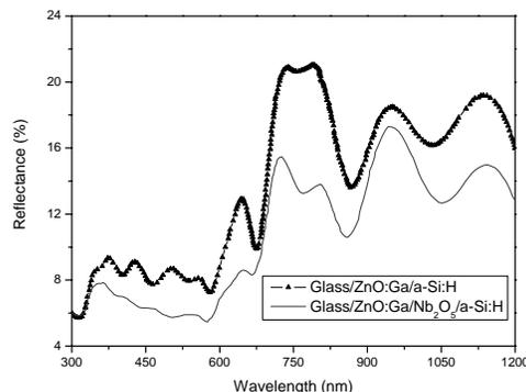
Fig. 2. Reflectance spectra of ZnO:Ga/a-Si:H coated glass with and without a ARL  $\text{Nb}_2\text{O}_5$ .
