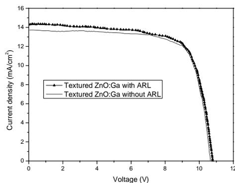
Fig. 3. J-V curves of a-Si:H solar cells fabricated on textured ZnO:Ga with and without ARL.
