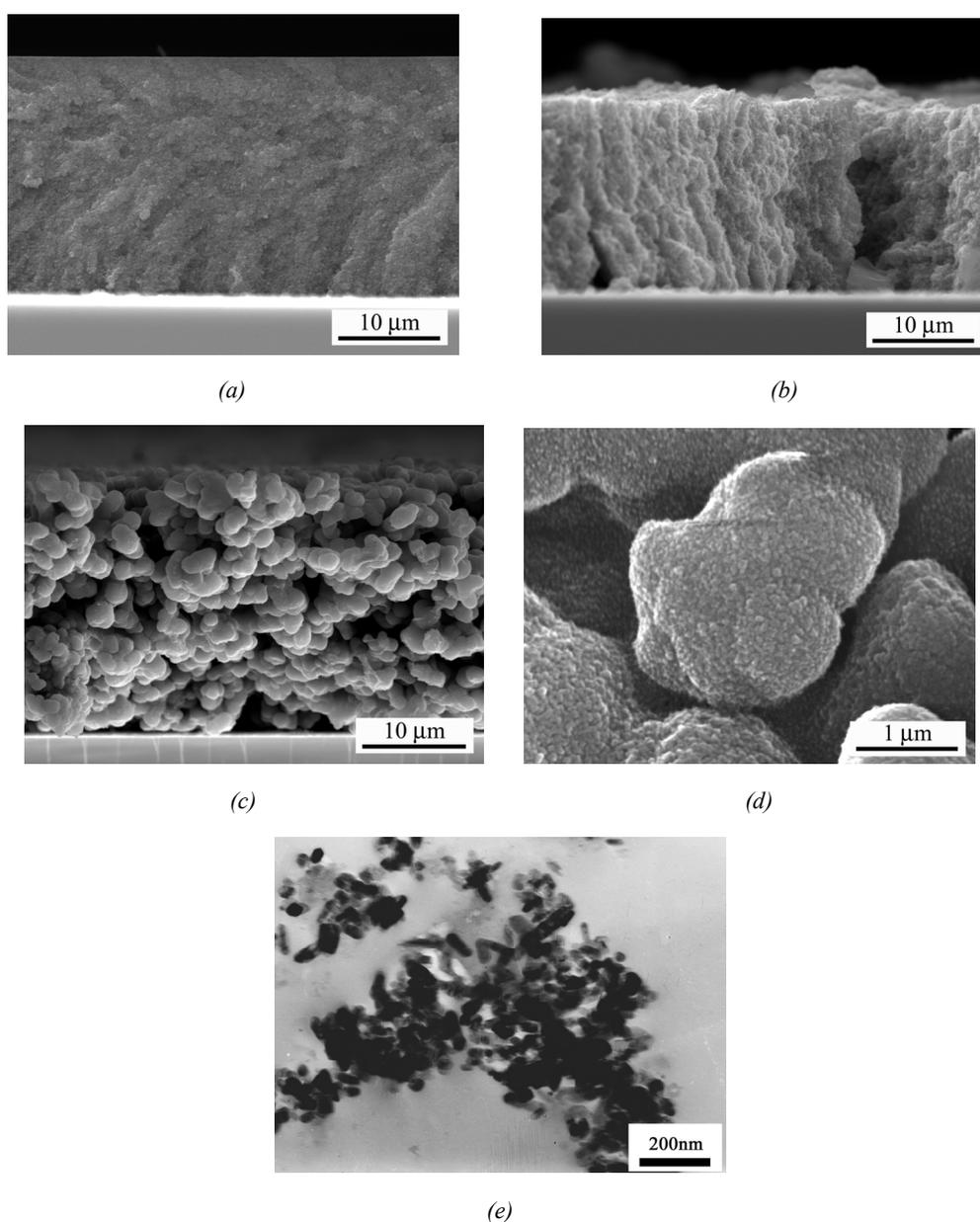
Fig. 1. SEM cross-sectional views of *SP-trans* (a) and *SP-op* (b) TiO<sub>2</sub> films, coral-like TiO<sub>2</sub> films at low magnification (c) and at high magnification (d), and TEM image of coral-like TiO<sub>2</sub> powder (e).
