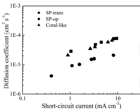
Fig. 5. The electron diffusion coefficient of the electrodes based on the *SP-trans* (square), *SP-op* (circle) and *coral-like* (triangle) TiO<sub>2</sub> films..
