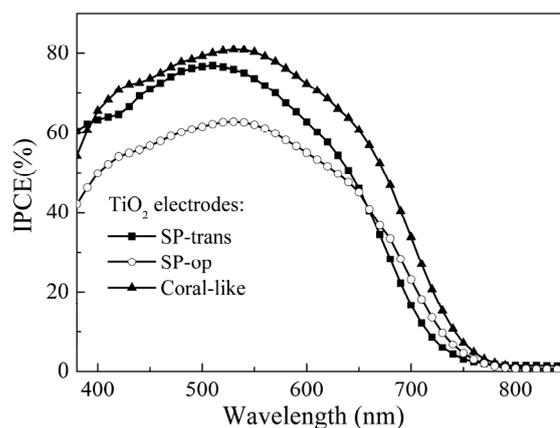
Fig. 4. IPCE spectra of DSSCs based on the *SP-trans* (solid square), *SP-op* (circle) and *coral-like* (solid triangle) TiO<sub>2</sub> films.
