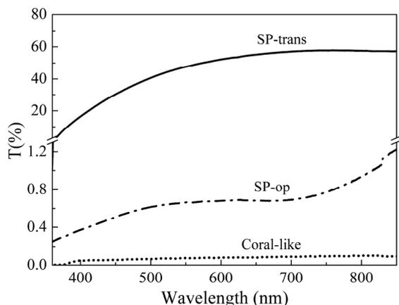
Fig. 2. Transmittance of 10- $\mu\text{m}$ -thick *SP-trans*, *SP-op* and *coral-like* TiO<sub>2</sub> films.
