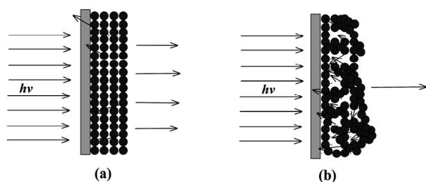
Fig. 3. Scheme of light scattering of *SP-trans* TiO<sub>2</sub> film (a) and *coral-like* TiO<sub>2</sub> film (b).
