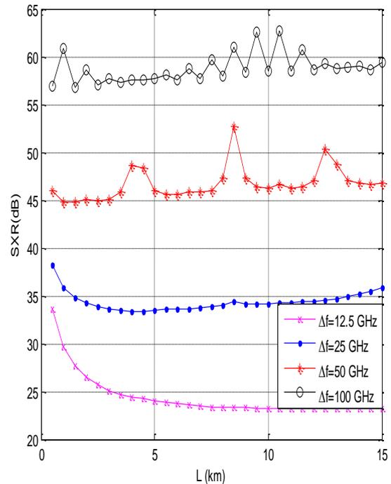
Fig. 10. Variation of SXR with varying channel lengths for center channels of 35-channel DWDM-GPON systems having 12.5 GHz, 25 GHz, 50 GHz and 100 GHz channel spacing values and 1 mW channel input powers
