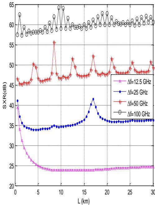
Fig. 8. Variation of SXR with varying channel lengths for center channels of 15-channel DWDM-GPON systems having 12.5 GHz, 25 GHz, 50 GHz and 100 GHz channel spacing values and 1 mW channel input powers
