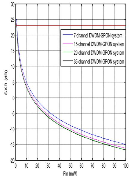
Fig. 2. Variation of SXR with channel input power variations for center channels of 7-, 15-, 29- and 35-channel DWDM-GPON systems for 12.5 GHz channel spacings
