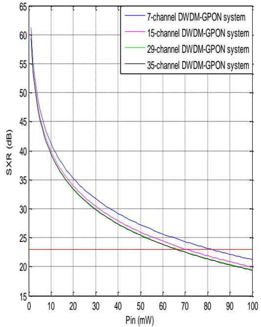
Fig. 5. Variation of SXR with channel input power variations for center channels of 7-, 15-, 29- and 35-channel DWDM-GPON systems for 100 GHz channel spacings
