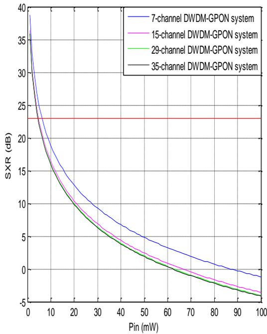
Fig. 3. Variation of SXR with channel input power variations for center channels of 7-, 15-, 29- and 35-channel DWDM-GPON systems for 25 GHz channel spacings
