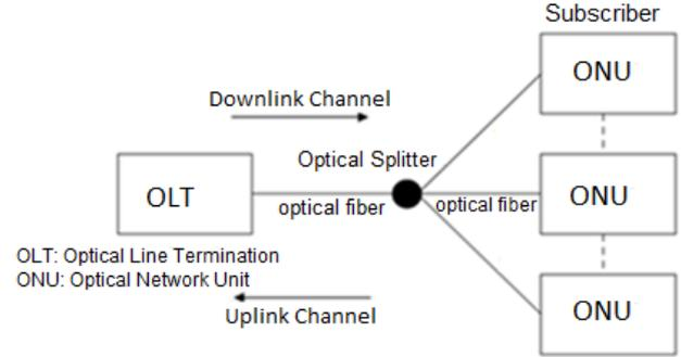
Fig. 1. Components of a PON
