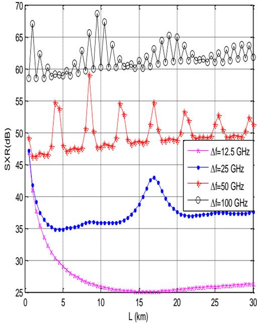
Fig. 7. Variation of SXR with varying channel lengths for center channels of 7-channel DWDM-GPON systems having 12.5 GHz, 25 GHz, 50 GHz and 100 GHz channel spacing values and 1 mW channel input powers
