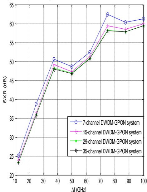
Fig. 6. Variation of SXR with variations in channel spacing values for center channels of 7-, 15-, 29- and 35-channel DWDM-GPON systems for 1 mW channel input powers
