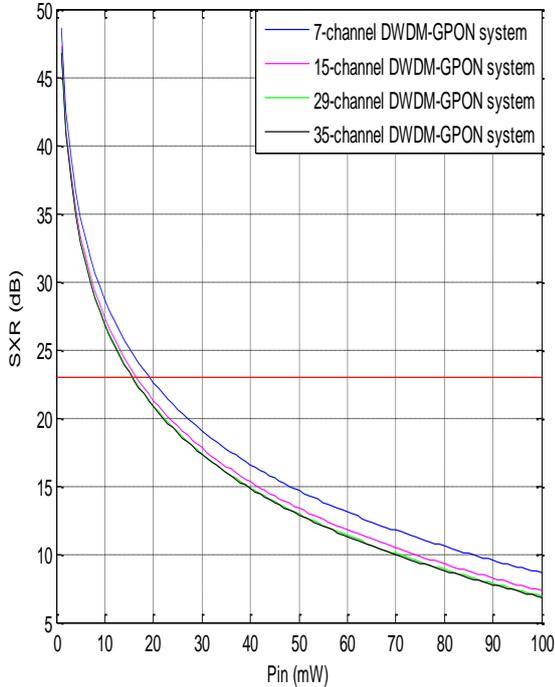
Fig. 4. Variation of SXR with channel input power variations for center channels of 7-, 15-, 29- and 35-channel DWDM-GPON systems for 50 GHz channel spacings
