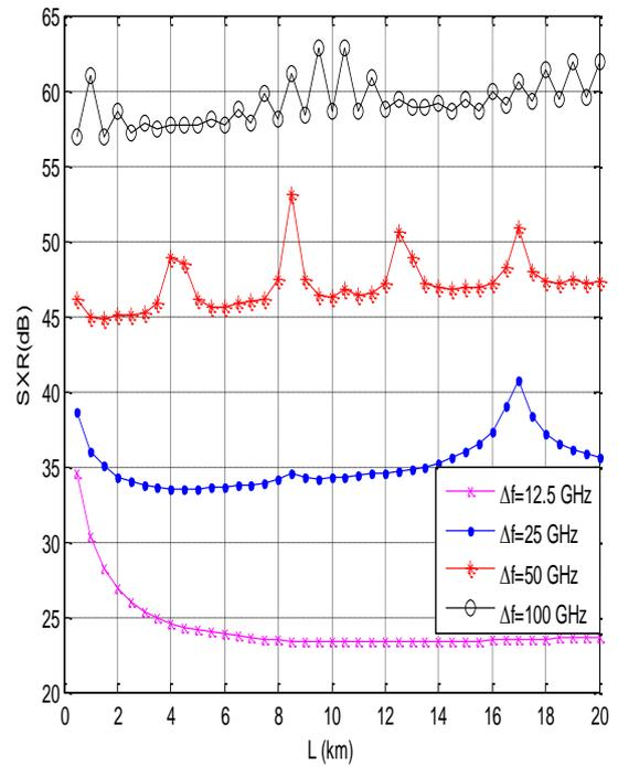
Fig. 9. Variation of SXR with varying channel lengths for center channels of 29-channel DWDM-GPON systems having 12.5 GHz, 25 GHz, 50 GHz and 100 GHz channel spacing values and 1 mW channel input powers
