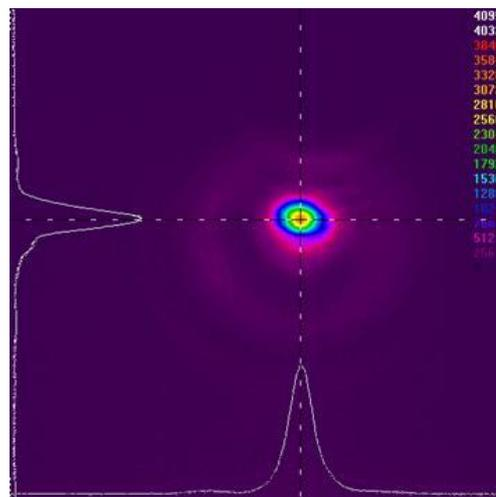
Fig. 4. The laser beam profile for passively Q-switched  $\text{YVO}_4/\text{Nd}:\text{YVO}_4$  laser at the maximum output power
