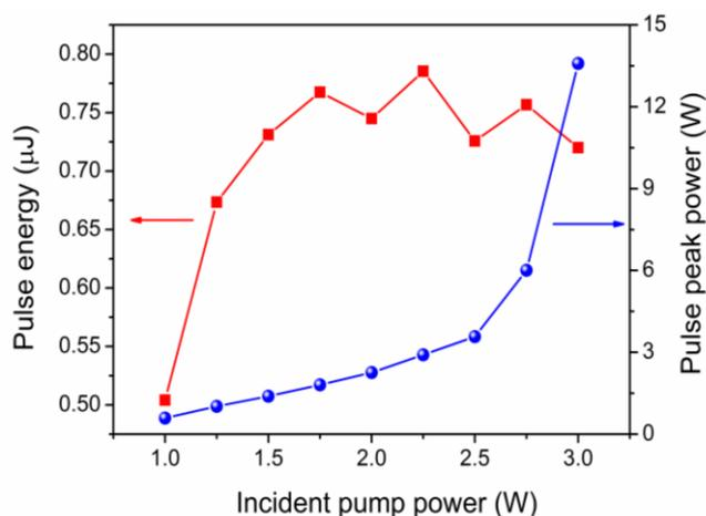
Fig. 6. Pulse energy and pulse peak power as a function of incident pump energy for passively Q-switched YVO<sub>4</sub>/Nd:YVO<sub>4</sub> laser
