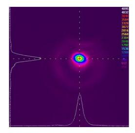
*Fig. 4. The laser beam profile for passively Q-switched YVO*<sub>4</sub>/*Nd*:*YVO*<sub>4</sub> *laser at the maximum output power*
