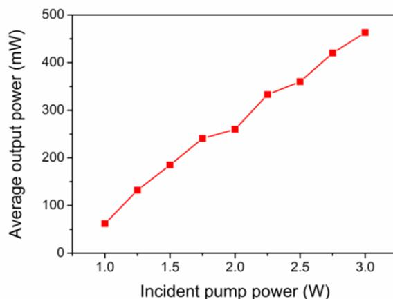
Fig. 3. Average output power as a function of incident pump power for passively Q-switched  $\text{YVO}_4/\text{Nd}:\text{YVO}_4$  laser
