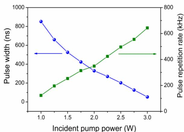
Fig. 5. Pulse width and pulse repetition rate as a function of incident pump energy for passively Q-switched YVO<sub>4</sub>/Nd:YVO<sub>4</sub> laser
