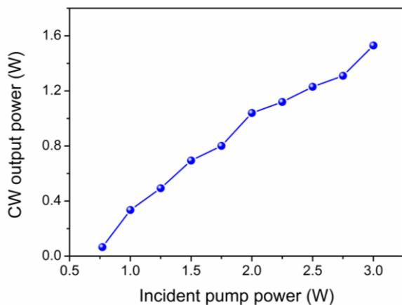
Fig. 2. CW output power as a function of incident pump power
