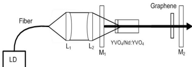
Fig. 1. Schematic of the passively Q-switched  $\text{YVO}_4/\text{Nd}:\text{YVO}_4$  laser
