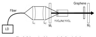
Fig. 1. Schematic of the passively Q-switched YVO4/Nd:YVO4 laser
