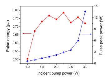
Fig. 6. Pulse energy and pulse peak power as a function of incident pump energy for passively Q-switched YVO4/Nd:YVO4 laser
