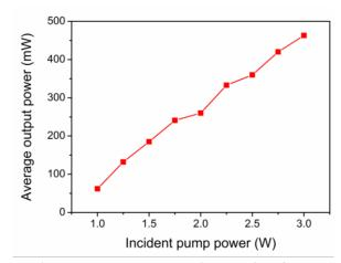
Fig. 3. Average output power as a function of incident pump power for passively Q-switched YVO<sub>4</sub>/Nd:YVO<sub>4</sub> laser
