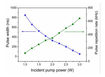
Fig. 5. Pulse width and pulse repetition rate as a function of incident pump energy for passively Q-switched YVO4/Nd:YVO4 laser
