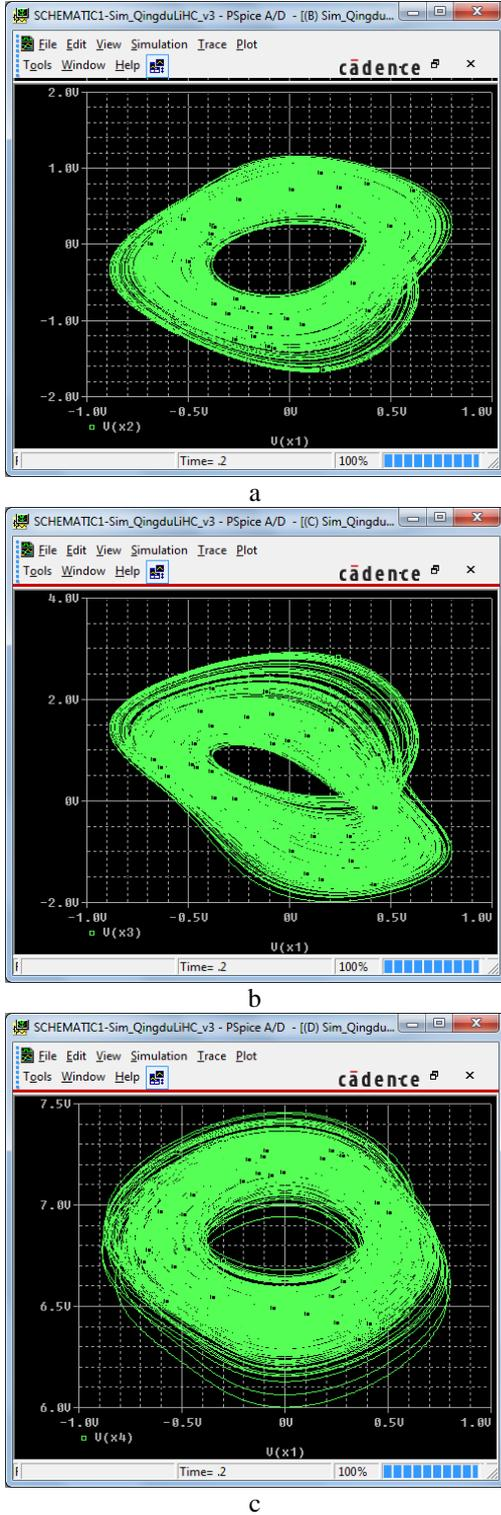
Fig. 9. Hyperchaotic attractor of the designed electronic circuit obtained from OrCAD (a) in the  $x_1 - x_2$  plane, (b) in the  $x_1 - x_3$  plane, and (c) in the  $x_1 - \phi$  plane.
