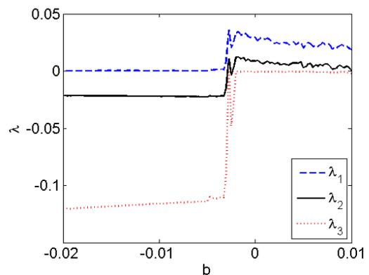
Fig. 5. Three largest Lyapunov exponents  $\lambda_1$ ,  $\lambda_2$ ,  $\lambda_3$  (blue dash line, black solid line, and red dot line, respectively) of network (5) versus  $b$  for  $a = -0.05$ .
