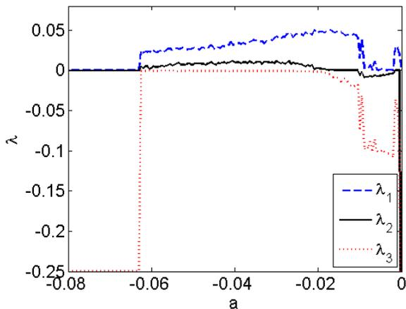
Fig. 7. Three largest Lyapunov exponents  $\lambda_1$ ,  $\lambda_2$ ,  $\lambda_3$  (blue dash line, black solid line, and red dot line, respectively) of neural network (5) versus  $a$  for  $b = -0.001$ .
