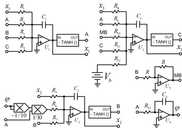
Fig. 8. Circuitual schematic of the proposed memristive neural network without equilibrium (5).
