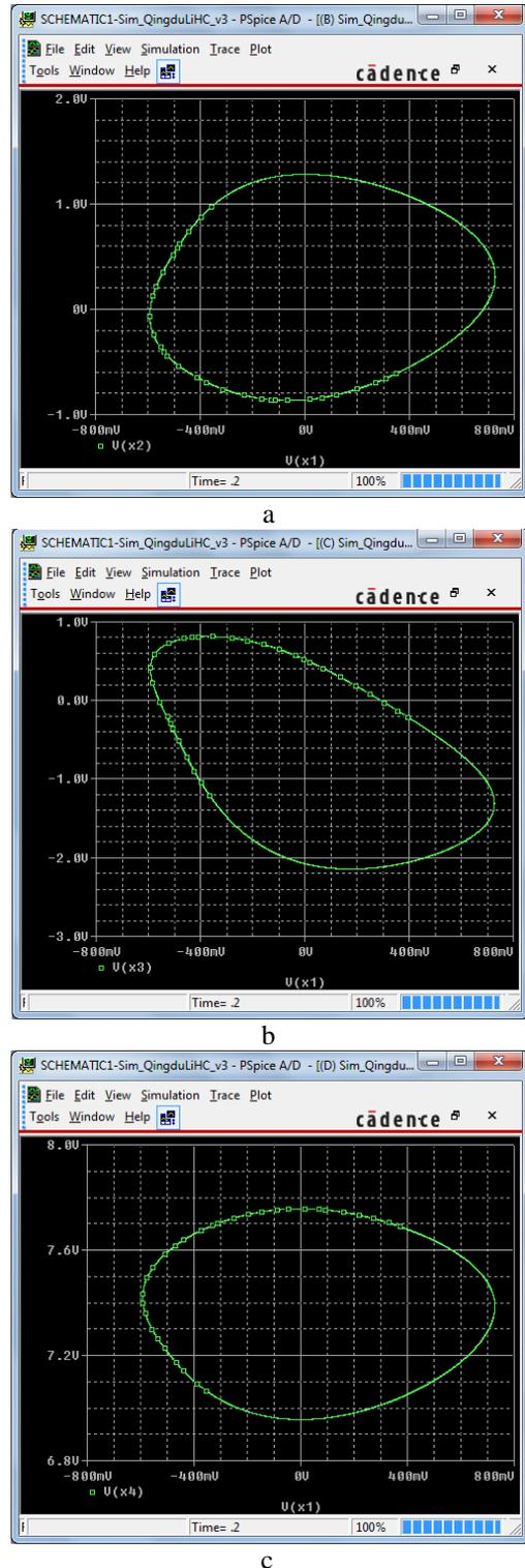
Fig. 10. The periodic orbit of the designed electronic circuit obtained from OrCAD (a) in the  $x_1 - x_2$  plane, (b) in the  $x_1 - x_3$  plane, and (c) in the  $x_1 - \phi$  plane.
