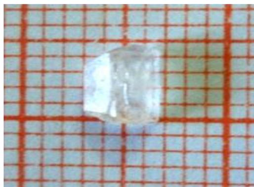
Fig. 2. Grown crystals of MAO.
