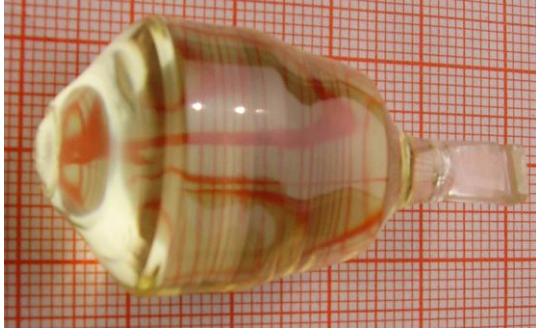
Fig. 1. Pr 3+ :Sr 3 La 2 (BO 3 ) 4 single crystal grown by the Czochralski method.
