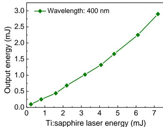
Fig. 6. Output energy of blue laser at 400 nm as a function of Ti:sapphire laser energy.
