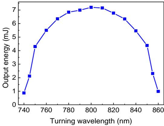
Fig. 2. Output energy as a function of laser wavelength at incident pump energy of 50 mJ
