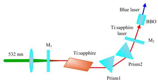
Fig. 1. Schematic of tunable Ti:Sapphire laser and frequency-doubling blue laser.
