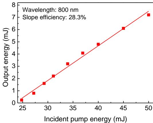
Fig. 3. Output energy as a function of incident pump energy at 800 nm.
