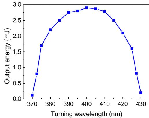
Fig. 5. Output energy for the tunable blue laser from 370 nm to 430 nm.
