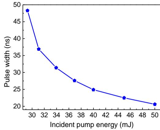
Fig. 4. Pulse width as a function of incident pump energy at 800 nm wavelength.
