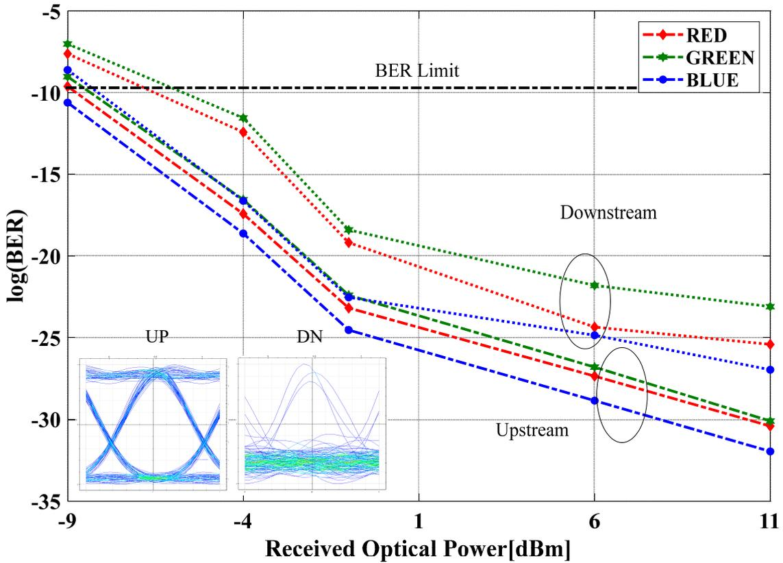
Fig. 5.  $\log(\text{BER})$  vs. received power of hybrid WDM-VLC-OCDMA PON; Insets: DN and UP eye patterns (color online)
