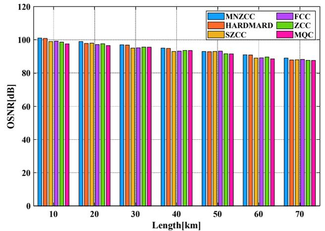
Fig. 6. OSNR(dB) Vs. fiber length of hybrid WDM-VLC-OCDAM PON (color online)
