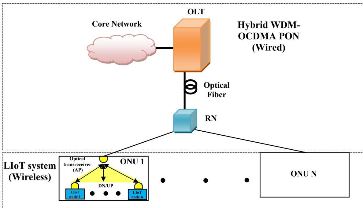
Fig. 1. Semantic diagram of an integrated OCDMA-WDM PON incorporating RGB LED based VLC system (color online)
