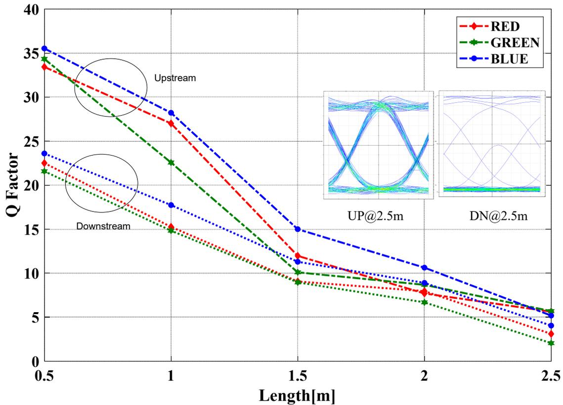
Fig. 3. Q-Factor vs. VLC length of the hybrid WDM-VLC-OCDAM PON; Insets: DN and UP eye patterns (color online)
