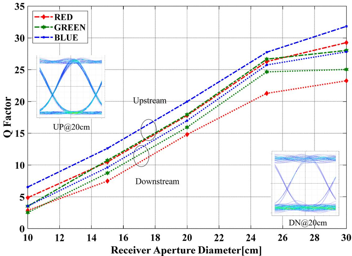
Fig. 4. *Q-Factor vs. aperture diameter at receive of hybrid WDM-VLC-OCDAM PON; Insets: DN and UP eye patterns (color online)*
