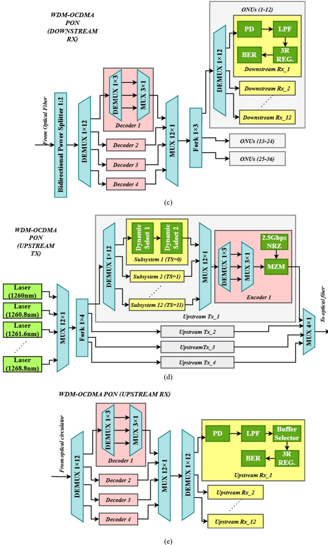
Fig. 2. (a) Conceptual diagram of full-duplex hybrid VLC-OCDMA-WDM PON utilizing MNZCC codes, (b) downstream transmitter section of OCDMA-WDM PON, (c) downstream receiver section of OCDMA-WDM PON, (d) upstream transmitter section of OCDMA-WDM PON and (e) upstream receiver section of OCDMA-WDM PON (color online)
