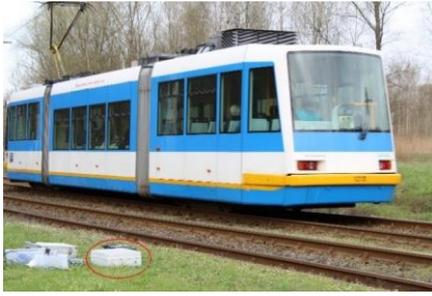
Fig. 7. A photo from the real measurement (red marked position of the interferometric sensor)
