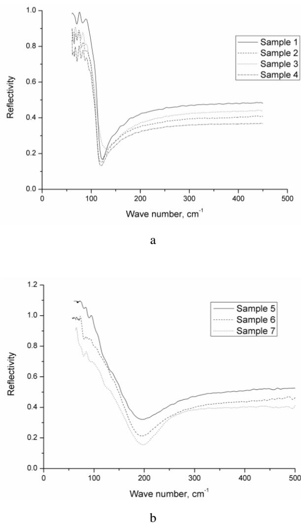
Fig. 1. Room temperature FIR diagrams for (a) samples (1-4): 1)  $Pb_{0.4614}Mn_{0.0167}Yb_{0.0048}Te_{0.517}$ ; 2)  $Pb_{0.465}Mn_{0.0179}Yb_{0.0073}Te_{0.5096}$ ; 3)  $Pb_{0.464}Mn_{0.0121}Yb_{0.0053}Te_{0.5184}$ ; 4)  $Pb_{0.4911}Mn_{0.0117}Yb_{0.0068}Te_{0.4913}$ ; (b) samples (5-7): 5)  $Pb_{0.461}Mn_{0.0034}Yb_{0.0025}Te_{0.533}$ ; 6)  $Pb_{0.46}Mn_{0.0015}Yb_{0.0095}Te_{0.528}$ ; 7)  $Pb_{0.466}Yb_{0.016}Te_{0.517}$ .
