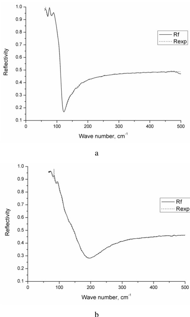
Fig. 2. Far infrared reflectivity spectrum of (a)  $Pb_{0.4614}Mn_{0.0167}Yb_{0.0048}Te_{0.517}$  (b)  $Pb_{0.461}Mn_{0.0034}Yb_{0.0025}Te_{0.533}$ . Experimental spectrum is presented by points while the full line was calculated using the fitting procedure.
