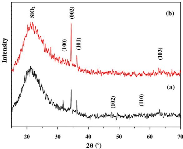
Fig. 2. XRD patterns of the five layers ZnO: Al films direct annealed at (a) 600 °C and (b) 700 °C.
