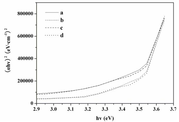
Fig. 5. Plots of  $(\alpha hv)^2$  vs.  $hv$  for ZnO: Al films (a) preannealed at 400 °C and annealed at 600 °C, (b) direct annealed at 700 °C, (c) preannealed at 400 °C and annealed at 700 °C, (d) annealed at 700 °C.
