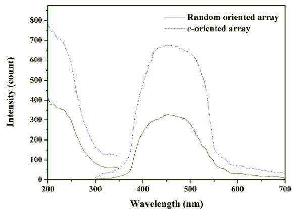
Fig. 6. Luminescence spectra of the ZnO: Al films annealed at 700°C.
