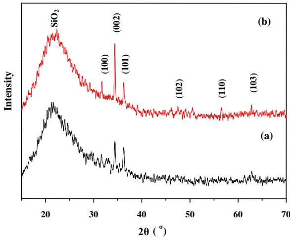
Fig. 1. XRD patterns of the five layers ZnO: Al films preheated at 400 °C and then annealed at (a) 600 °C and (b) 700 °C.
