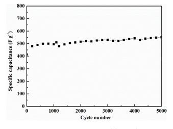
Fig. 5. Capacitance retention of the sample  $CoSe_2/C-900^{\circ}C$  at 10 A g<sup>-1</sup>
