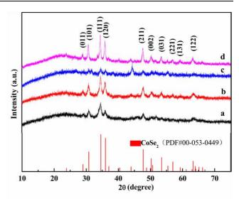
Fig. 1. XRD patterns of the CoSe<sub>2</sub>/carbonized foam composites obtained at different temperature. A, b, c and d represent the CoSe<sub>2</sub>/C-700 °C, CoSe<sub>2</sub>/C-800 °C, CoSe<sub>2</sub>/C-900 °C and CoSe<sub>2</sub>/C-1000 °C, respectively (color online)
