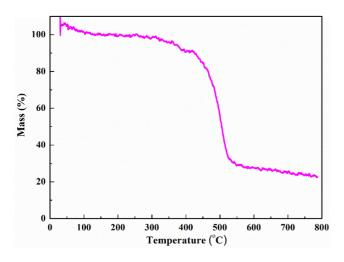
Fig. 3. TGA curve of the sample CoSe<sub>2</sub>/C-900 °C (color online)
