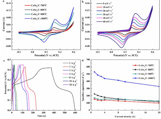
Fig. 4. (a) CV curves of the CoSe<sub>2</sub>/carbonized foam composites obtained at different temperature at 30 mV s<sup>-1</sup>, (b) CV curves of the sample CoSe<sub>2</sub>/C-900 °C, (c) GCD curves of the sample CoSe<sub>2</sub>/C-900 °C, (d) Specific capacitance of the CoSe<sub>2</sub>/carbonized foam composites obtained at different temperature (color online)
