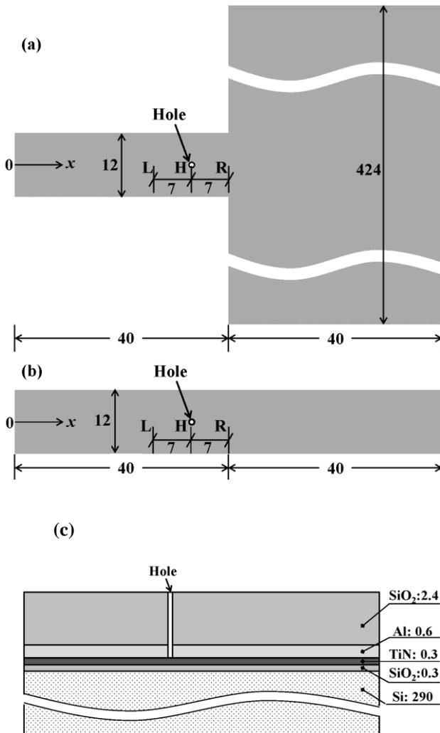
Fig. 1. Schematic illustration of samples [unit:  $\mu\text{m}$ ]. (a) Planar view of sample with sudden change in geometrical shape. (b) Planar view of sample without geometrical change. (c) Cross-sectional view of samples.
