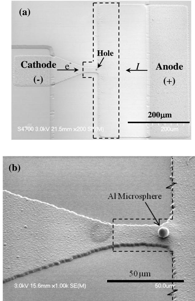
Fig. 2. FE-SEM images of the sample with a sudden change in geometrical shape, where the dashed lines enclose the sample shown in Fig. 1a. (a) Experimental sample. (b) Formation of Al microsphere at the predefined location.
