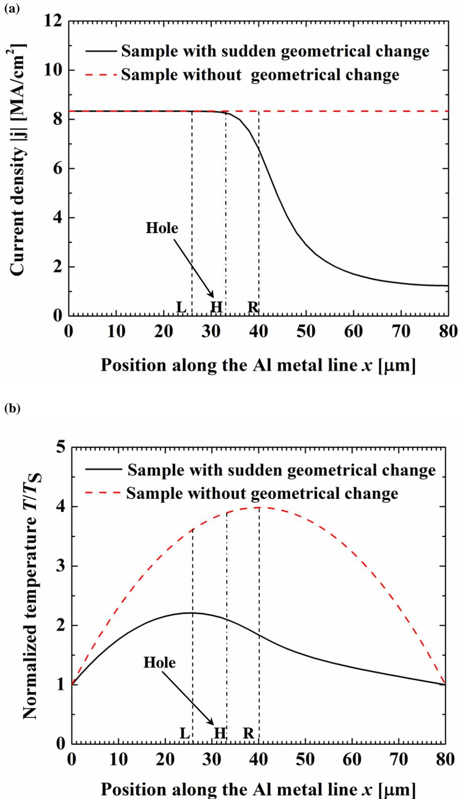
Fig. 3. 2D-FEA results of samples. (a) Current density distribution. (b) Temperature distribution.
