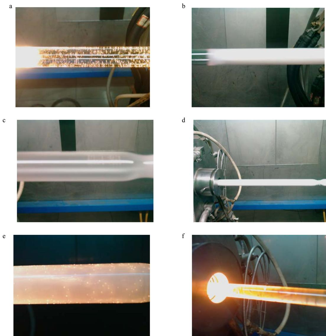
Fig. 4. Six main states of the fabrication process of perform. (a) Polishing and deposition of barrier layers. (b) Deposition of porous layer. (c) The thin film status after solution-doped. (d) Dehydration. (e) Vitrification. (f) Tube collapse.
