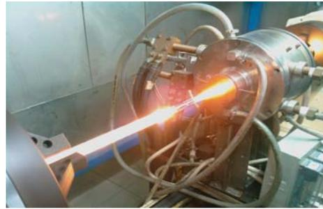
Fig. 3. The modified MCVD lathe with a carbon furnace in our laboratory.
