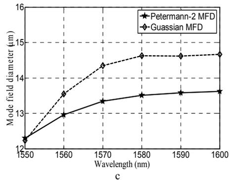
Fig. 6. The results were tested by PK2200. (a) This is the absorption spectra of the EDF, and the absorption peak is 19dB/m @ 1530nm. (b) The cutoff wavelength is 1176nm. (c) The relationship between MFD and wavelength. Actually, there are two curves, because the instrument produces the MFD according to Petermann-2 and Gaussian definitions.
