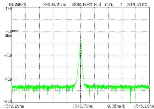
Fig. 10. Output spectrum of the EDFL, a stable and narrow-band peak is observed.
