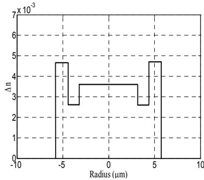
Fig. 1. Schematic diagram of refractive index profile of one kind of LMA EDF.
