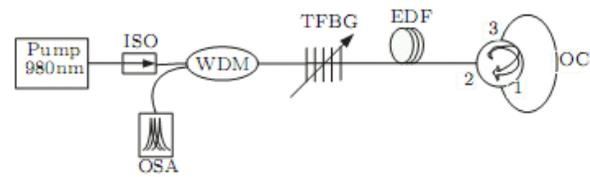
Fig. 8. Configuration of the linear-cavity EDFL based on TFBG and OC.
