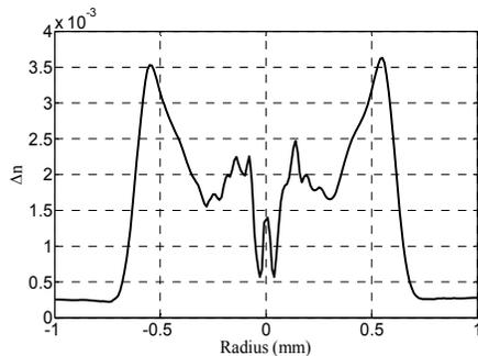
Fig. 5. The refractive index profile of the self-made perform.
