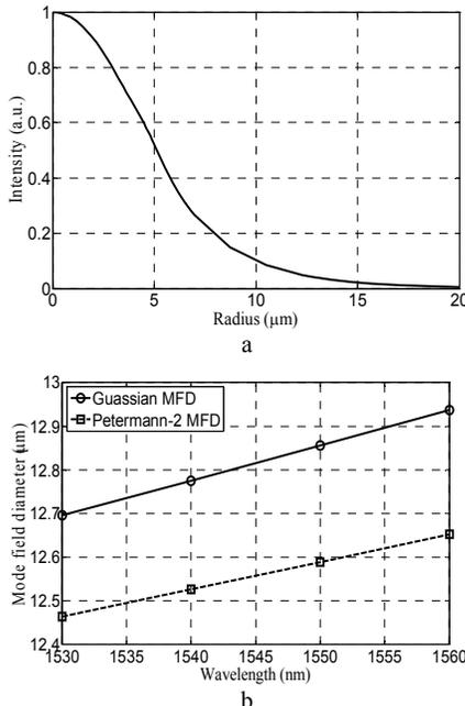
Fig. 2. The MFD specifications of the fiber. (a) The distribution of the MFD. (b) The MFD vs. wavelength.
