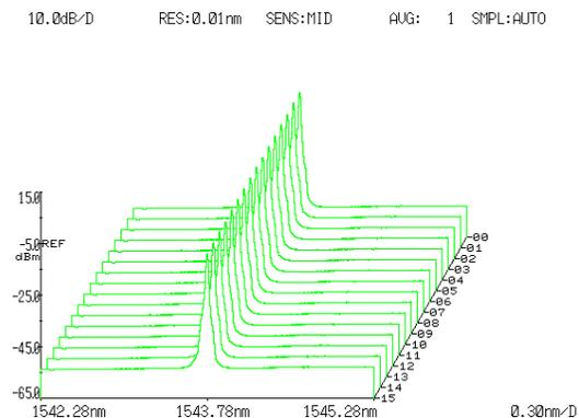
Fig. 11. The 16-time repeated scan of lasing spectra over 15 min.
