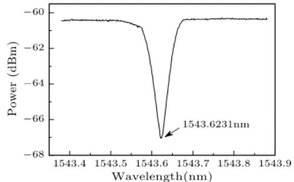
Fig. 9. Original transmission spectrum of TFBG.
