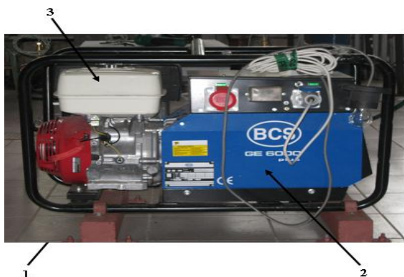
Fig. 2. Generator group left view: 1-engine, 2-generator, and 3-tank.
