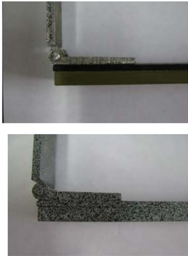
Fig. 2. Piezoelectric composite specimen and the applied speckle pattern.
