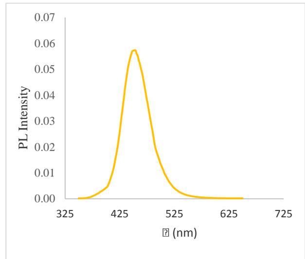
Fig. 3. Room temperature PL spectra of Ag-doped ZnS
