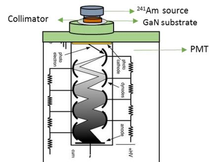
Fig. 1. The experimental set-up for testing the response of GaN
