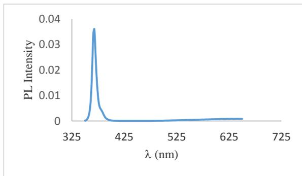
Fig. 2. Room temperature PL spectra of Si-doped GaN
