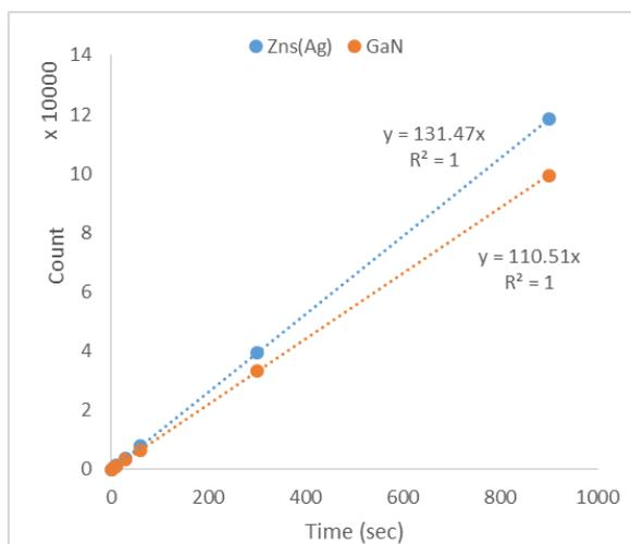
Fig. 5. Exposure time response of GaN & ZnS(Ag)
