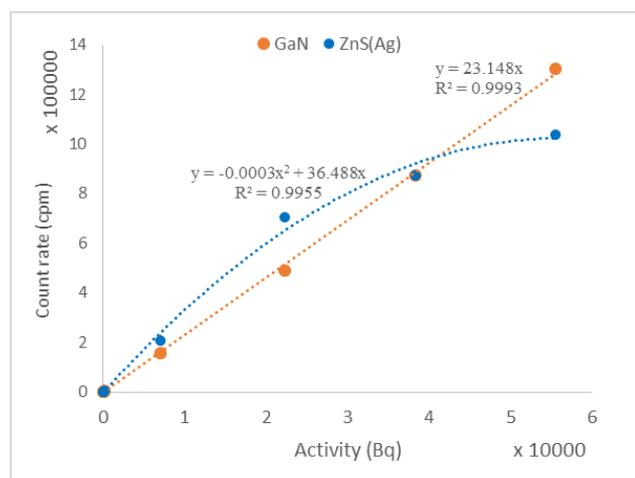
Fig. 6. GaN(Si) and ZnS(Ag) radioactivity dependence
