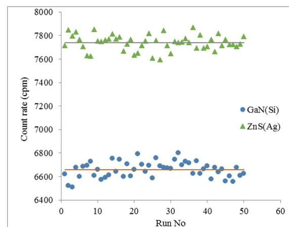
Fig. 4. Repeatability test for GaN and ZnS detectors
