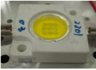
Fig. 1. The experimental WLED having CCT of 8500 K
