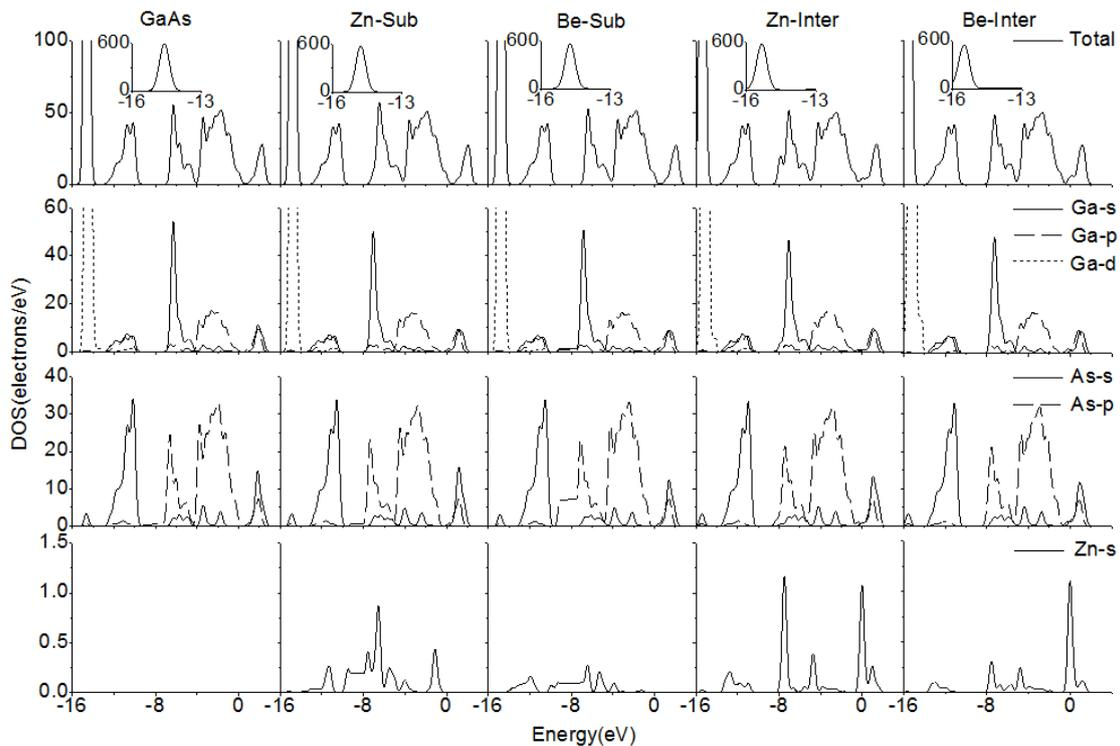
Fig. 2. DOS curves of intrinsic GaAs, Zn-Sub, Be-Sub, Zn-Inter and Be-Inter models
