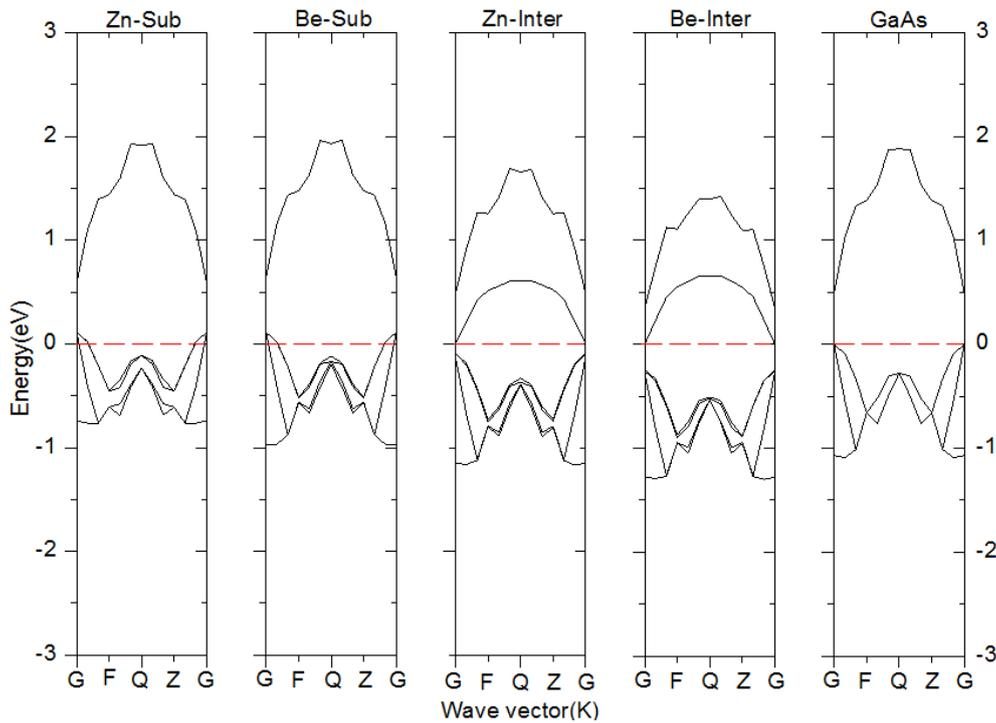
Fig. 1. Band structure of intrinsic GaAs, Zn-Sub, Be-Sub, Zn-Inter and Be-Inter models
