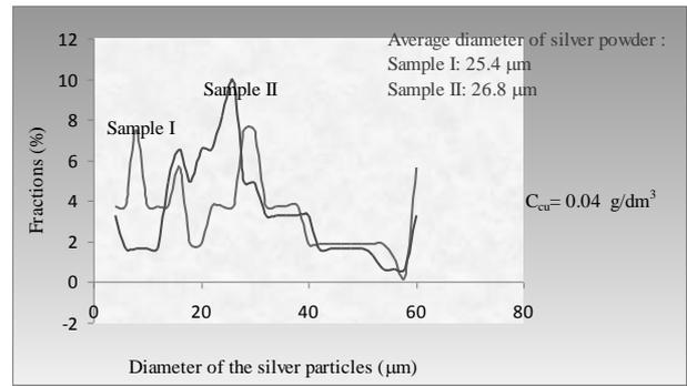
Fig. 9. Sedimentation curve of the silver powder analysis for  $C_{(Cu)}=0.04 \text{ g/dm}^3$  (II experiment).
