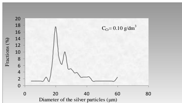
Fig. 14. Sedimentation curve of the silver powder analysis for  $C_{Cr} = 0.10 \text{ g/dm}^3$ .
