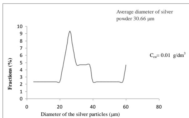
Fig. 4. Sedimentation curve of the silver powder analysis for  $C_{(\text{Cu})}=0.01 \text{ g/dm}^3$  (I experiment).
