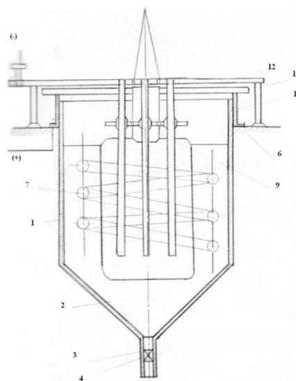
Fig. 2. Electrolytic cell with the cathode in the form of rods.
