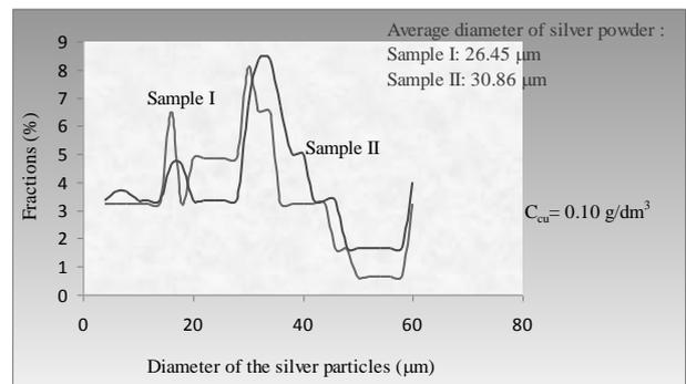
Fig. 12. Sedimentation curve of the silver powder analysis for  $C_{(Cu)}=0.10 \text{ g/dm}^3$  (II experiment).
