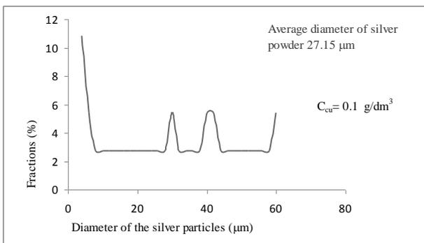
Fig. 6. Sedimentation curve of the silver powder analysis for  $C_{(Cu)}=0.1 \text{ g/dm}^3$  (I experiment).
