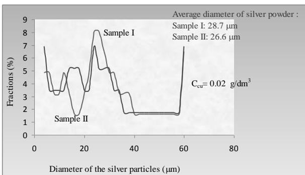
Fig. 8. Sedimentation curve of the silver powder analysis for  $C_{(Cu)}=0.02 \text{ g/dm}^3$  (II experiment).
