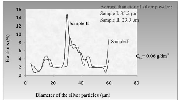
Fig. 10. Sedimentation curve of the silver powder analysis for  $C_{(Cu)}=0.06 \text{ g/dm}^3$  (II experiment).
