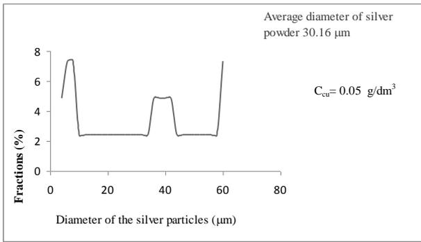
Fig. 5. Sedimentation curve of the silver powder analysis for  $C_{(Cu)}=0.05 \text{ g/dm}^3$  (I experiment).
