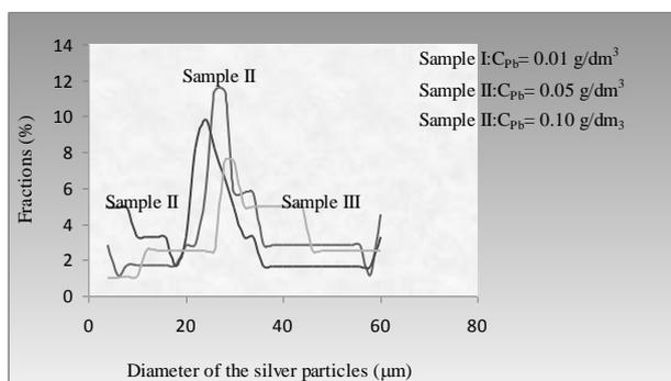
Fig. 13. Sedimentation curve of the silver powder analysis for various concentrations of  $Pb^{2+}$ .
