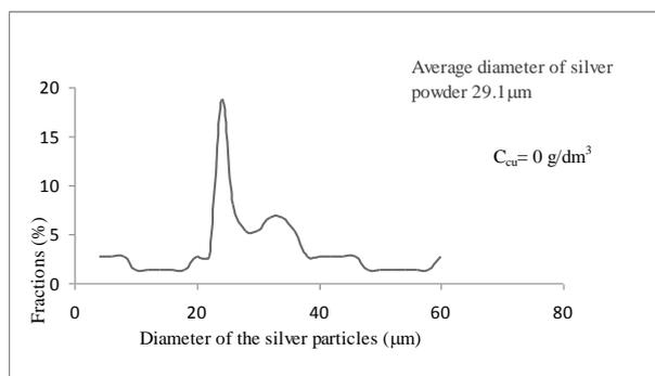
Fig. 3. Sedimentation curve of the silver powder analysis for  $C_{(\text{Cu})}=0 \text{ g/dm}^3$  (I experiment).
