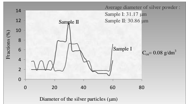
Fig. 11. Sedimentation curve of the silver powder analysis for  $C_{(Cu)}=0.08 \text{ g/dm}^3$  (II experiment).
