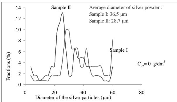
Fig. 7. Sedimentation curve of the silver powder analysis for  $C_{(Cu)}=0 \text{ g/dm}^3$  (II experiment).
