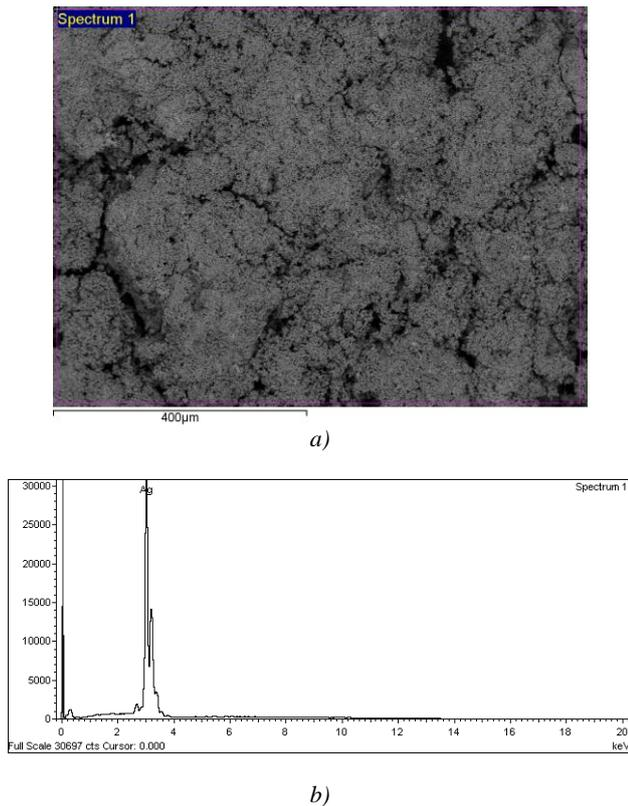
Fig. 19. EDS image with EDS spectrum of silver powder obtained at  $C_{Pb^{2+}} = 0.1 \text{ g/dm}^3$ : a) EDS image, b) EDS spectrum.
