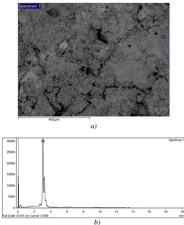
Fig. 20. EDS image with EDS spectrum of silver powder obtained at  $C_{Cr^{2+}} = 0.1 \text{ g/dm}^3$ : a) EDS image, b) EDS spectrum.
